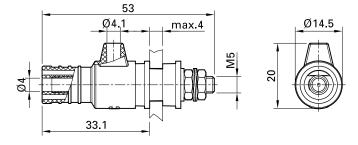
Insulated, with Ø 4 mm rigid socket accepting spring-loaded Ø 4 mm plugs with rigid insulating sleeve. Ø 3.2 mm cross hole for quick wire connection. Brass. The binding post is screwed into pre-drilled panels of plastic, metal, etc.Connection: Threaded bolt M5.
