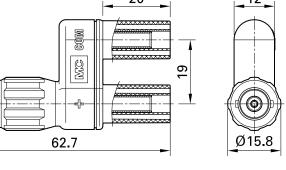
Two-pole touch-protected adapters with Ø 4 mm connectors linked to the BNC system. Version with BNC female connector and rigid Ø 4 mm sockets with rigid insulating sleeve. The contact sockets of the inner conductor of the BNC plug connector are in gold-plated brass.
