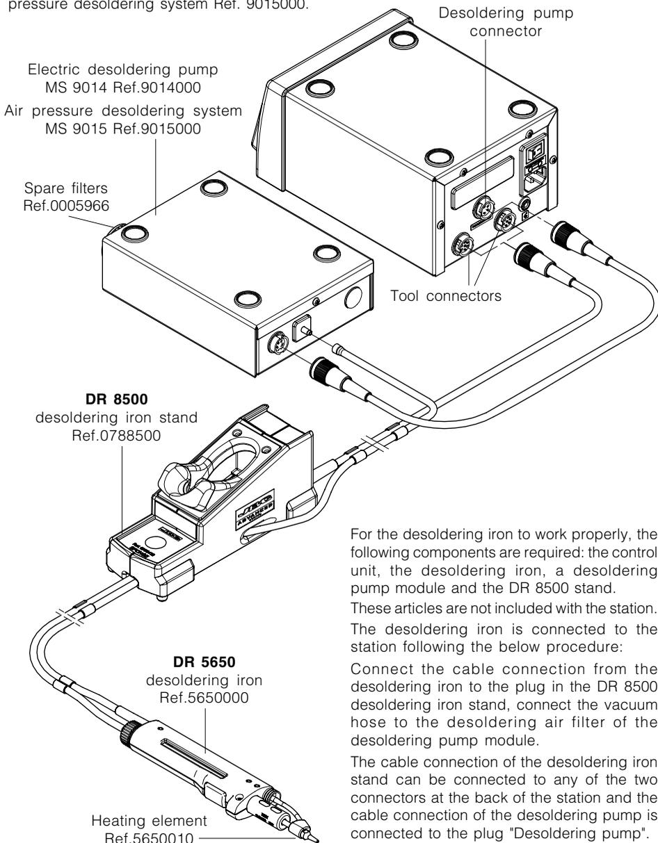
For the desoldering iron to work properly, the following components are required: the control unit, the desoldering iron, a desoldering pump module and the DR 8500 stand.
