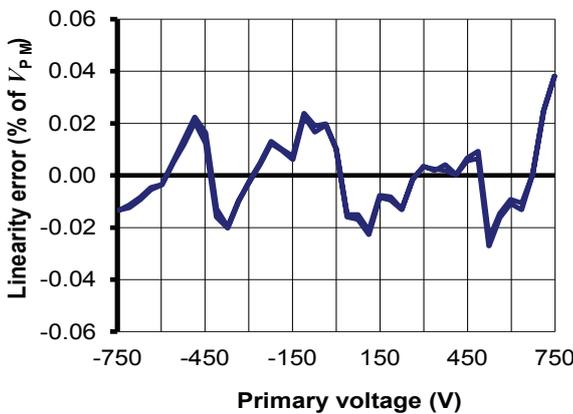
Figure 15: Typical linearity error at 25 °C
