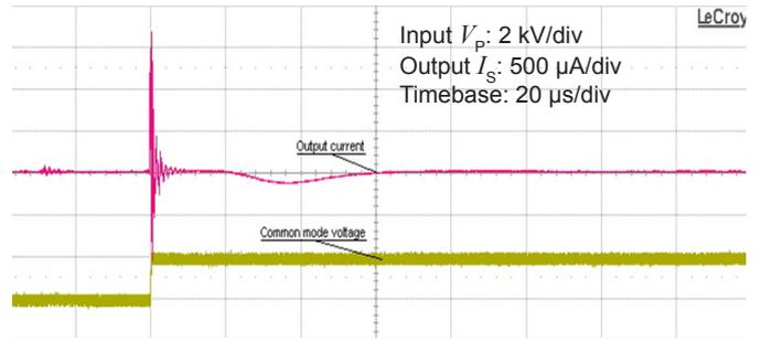
Figure 12: Detail of typical common mode perturbation (2000 V step with 6 kV/μs,  $R_M = 100 \Omega$ )
