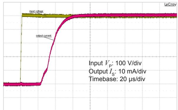
Figure 6: Typical step response (0 to 500 V)
