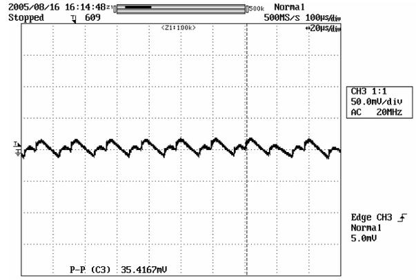
**Figure 24** – Ripple, 115 VAC, Full Load.
