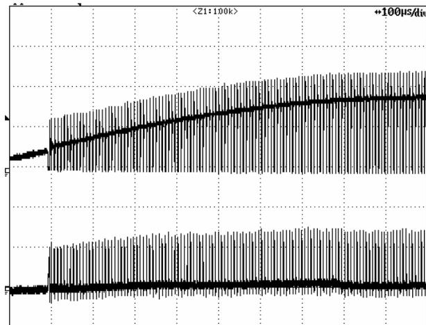
**Figure 19** – 265 VAC Input and Maximum Load.
