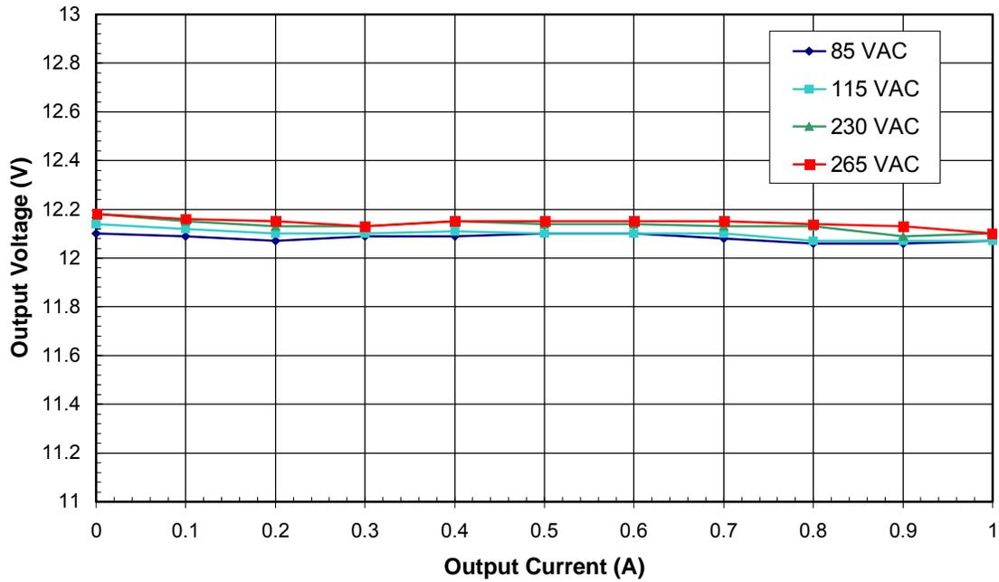
Figure 10 – Load and Line Regulation, Room Temperature.
