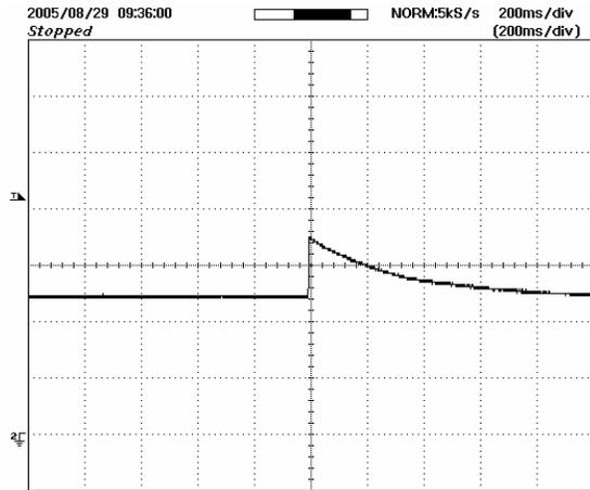
**Figure 25** – Overvoltage Shutdown.
