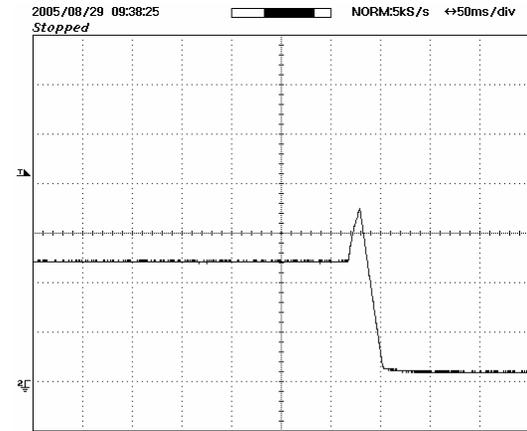
**Figure 26** – Overvoltage Shutdown.
