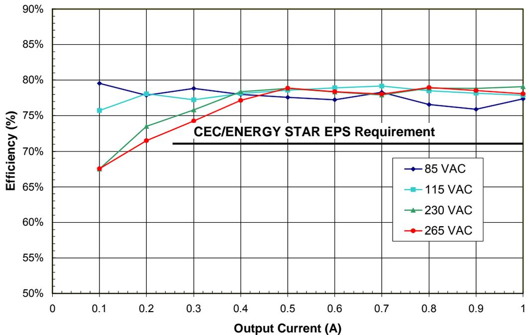
Figure 6 – Efficiency vs. Output Current, Room Temperature, 60 Hz.
