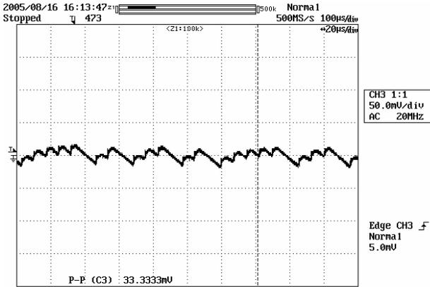
**Figure 23** – Ripple, 85 VAC, Full Load.
