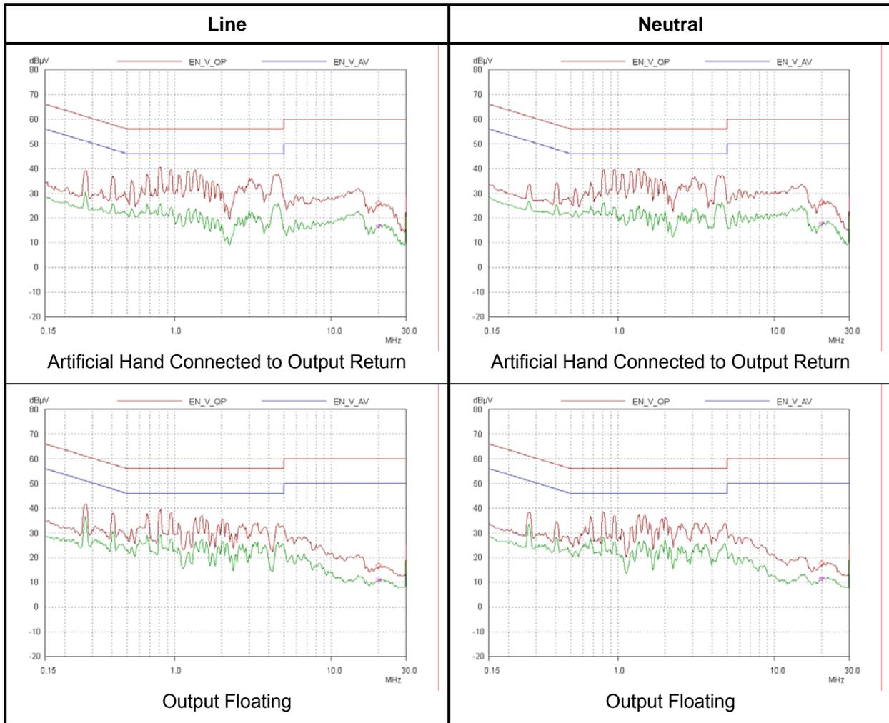
Figure 28 – Conducted EMI at 230 VAC.
