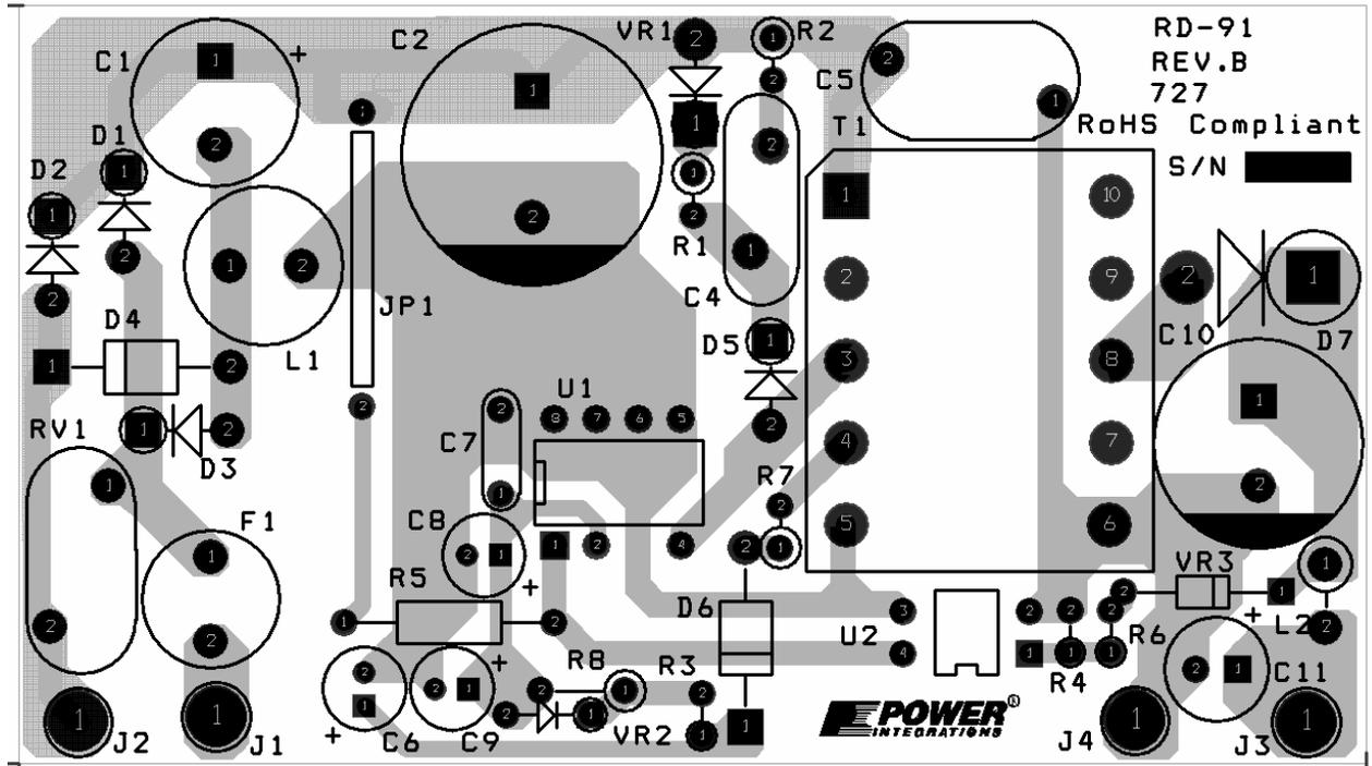
Figure 3 – Printed Circuit Board Layout (3.2 × 1.8 inches).
