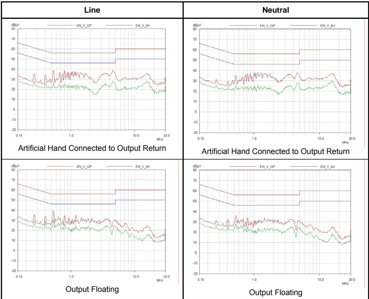
Figure 27 – Conducted EMI at 115 VAC.
