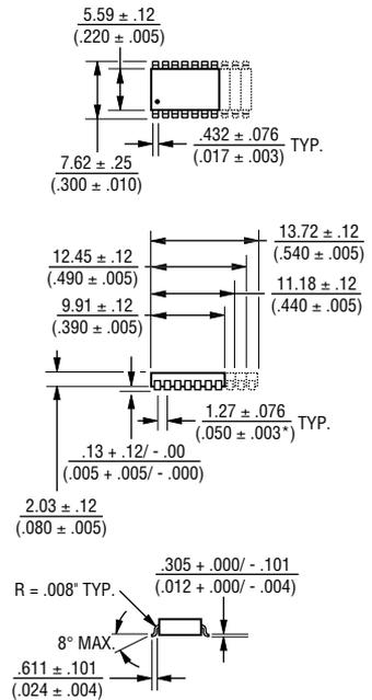
Lead coplanarity .102mm (.004 inch) max. at mounting surface.
