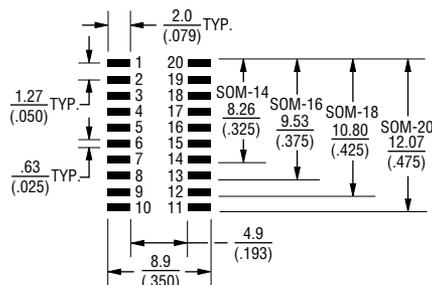
NOTE: Land pattern dimensions are based on  $\square$  design rules established by the Institute for Inter- $\square$  connecting and Packaging Electronic Circuits in  $\square$  IPC-SM-782.
