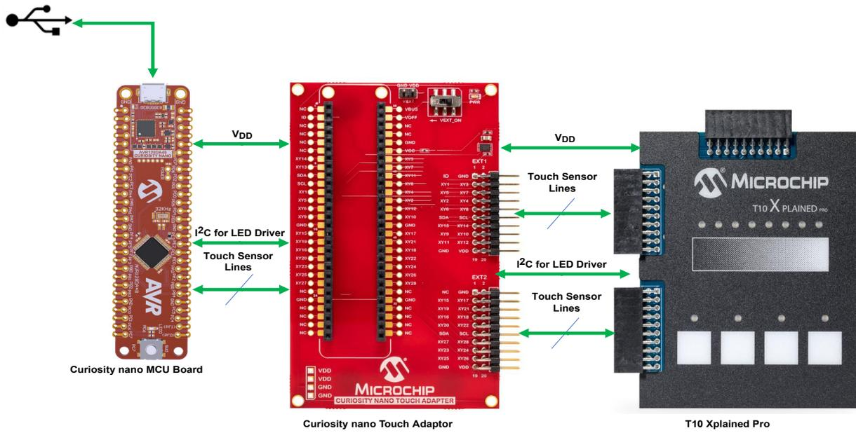
**Note:** All the above kits have on-board programmers/debuggers, which creates a set of low-cost boards for evaluation and demonstration of features and capabilities of different Microchip products.
