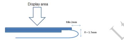
(12) The module should be fixed balanced into the housing, or the module may be twisted.
