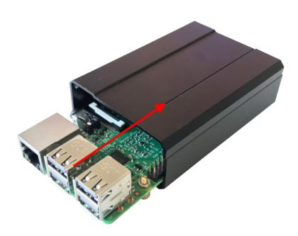
3. Screw the Raspberry Pi tight on the underside.
