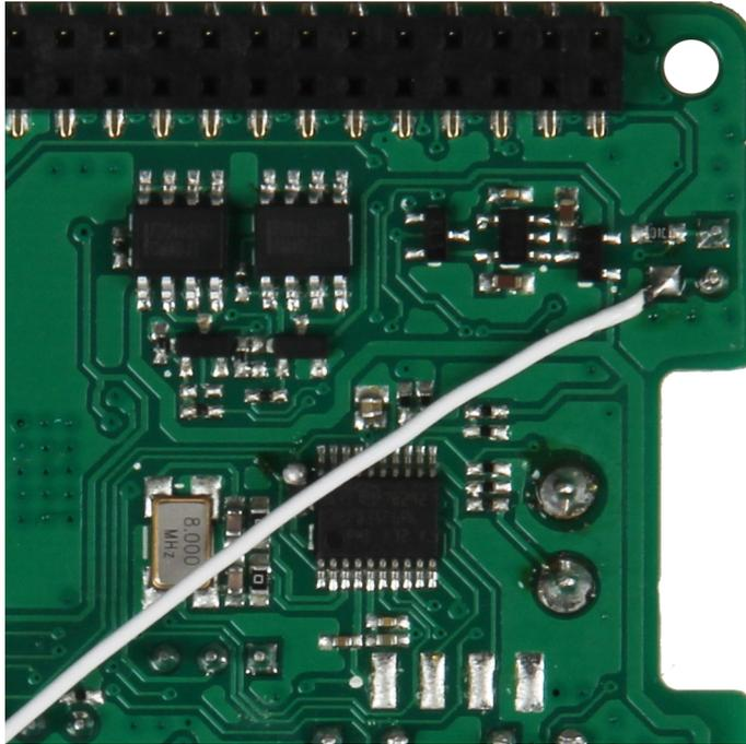
Solder the other end of the cable as shown in the picture below to one of the GPIO pins.
