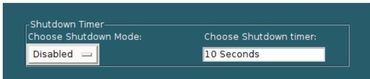
To enable the Shutdown Timer, select **Enable** at **Choose Shutdown Mode** and enter the desired shutdown time in seconds into the adjacent field. Finally, confirm with **Update**.
