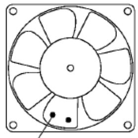
Note: The glues on the impeler is for impeler balance. Please don't remove it.
