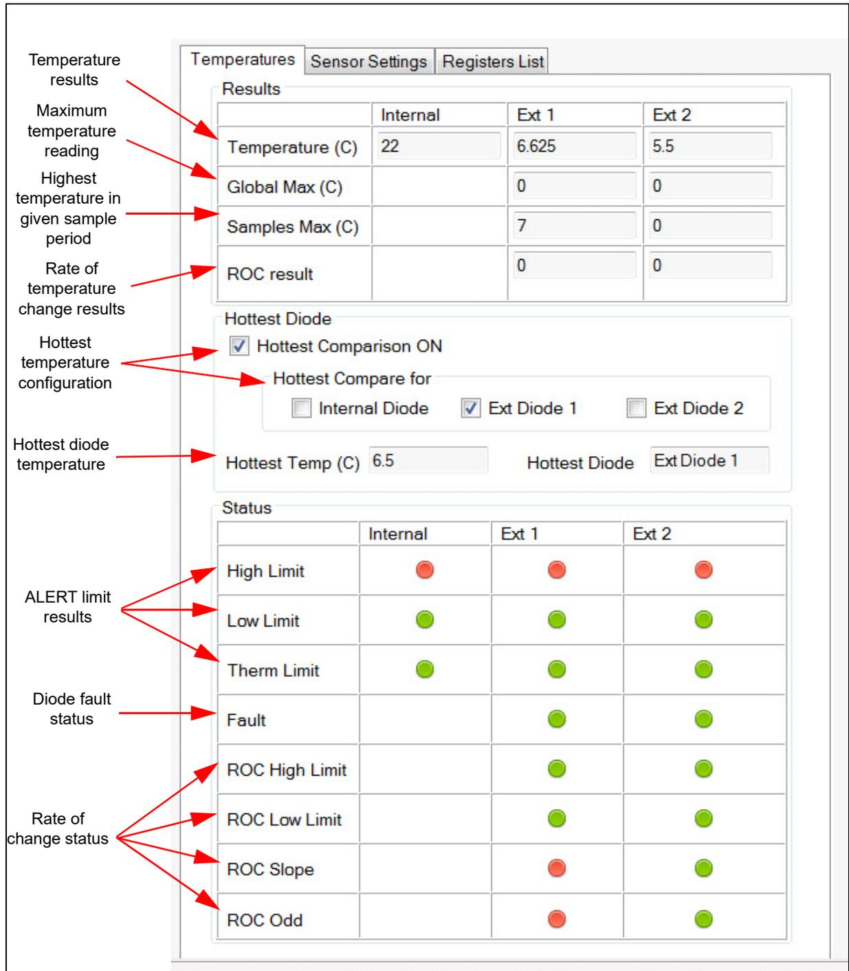
**FIGURE 3-4:** Temperatures Tab.
