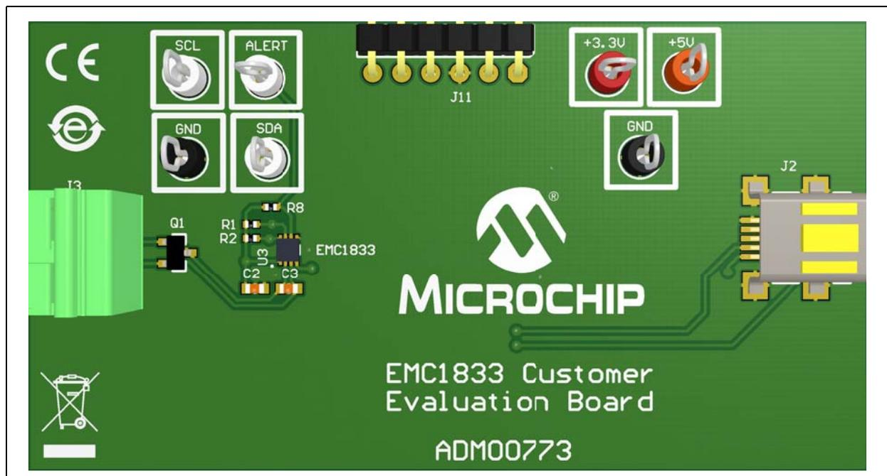
**FIGURE 1-1:** EMC1833 Evaluation Board (ADM00773) - Top View.
