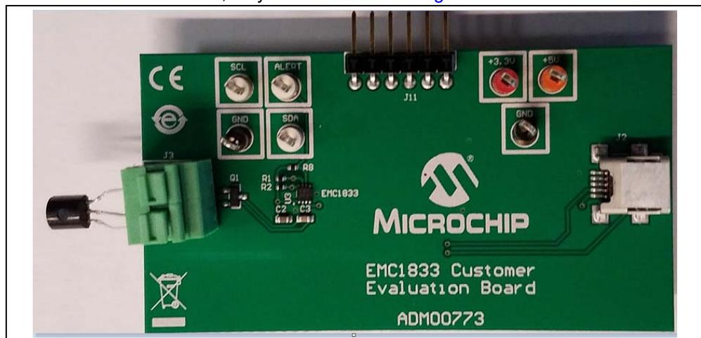
**FIGURE 2-1:** Board Connections.
