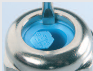
Fig. 3 With a large cable diameter – remove inlet. Insert screwdriver vertically into separating seam
