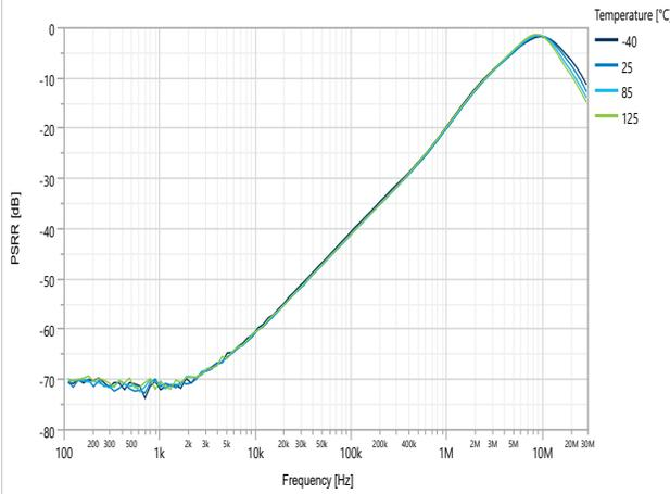
**Figure 49-104.** PSRR at DC and  $V_{CM} = V_{DD}/2$  over  $V_{DD}$  and Temperature
