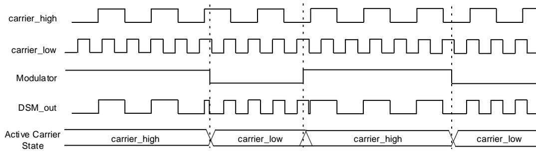
**Figure 33-6.** Full Synchronization (CHSYNC = 1, CLSYNC = 1)
