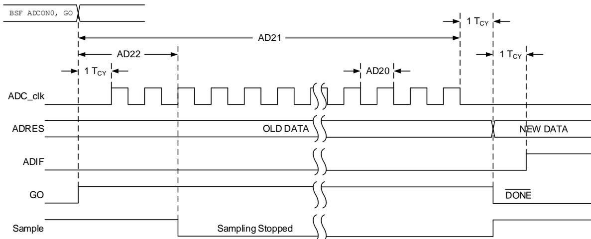
Figure 48-10. ADC Conversion Timing (ADC Clock from ADCRC)
