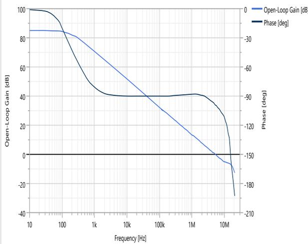
**Figure 49-106.** Open Loop Gain at 25°C over  $V_{DD}$  and  $V_{CM}$
