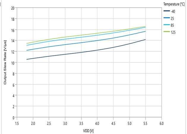
**Figure 49-109. Slew Rate Rise Time over  $V_{DD}$  and Temperature**
