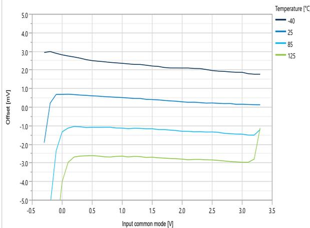
**Figure 49-102.** Input Offset Voltage at 5V over  $V_{CM}$  and Temperature
