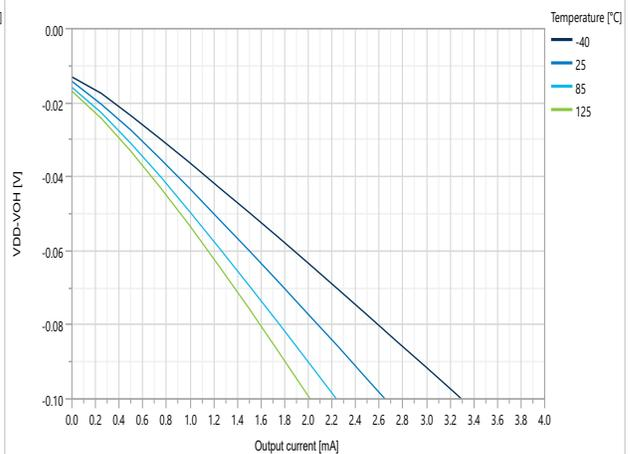
**Figure 49-111.**  $V_{OH}$  at 5V over Temperature and Load Current
