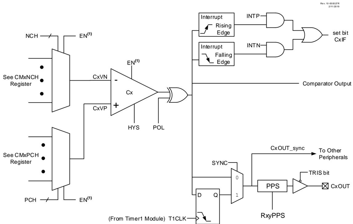
**Note 1:** When EN = 0, all multiplexer inputs are disconnected and the Comparator will produce a '0' at the output.
