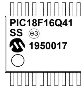
20-Lead SOIC (7.50 mm)
