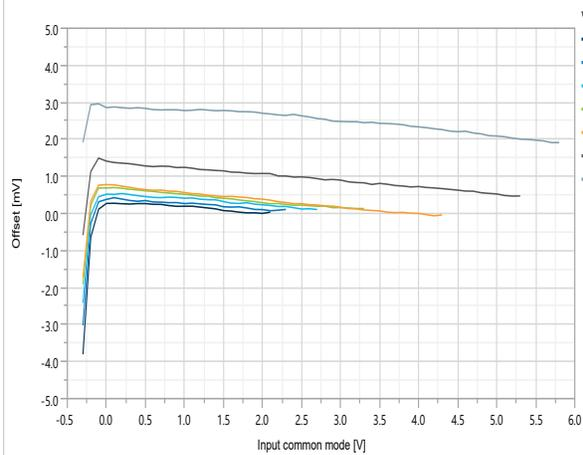
**Figure 49-100.** Input Offset Voltage at 25°C over  $V_{CM}$  and  $V_{DD}$  (CPON = 1)
