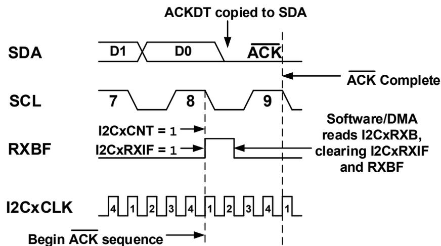
Figure 36-34. Not Acknowledge (NACK) Sequence Timing
