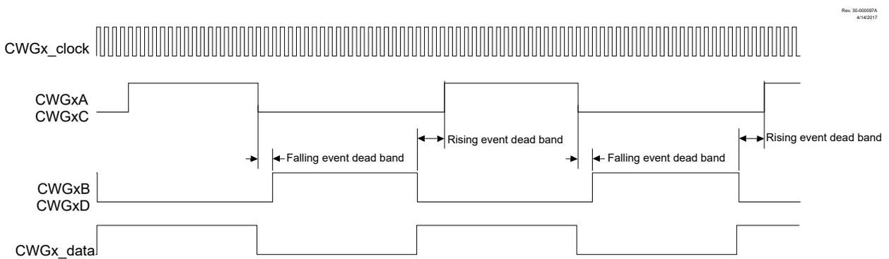
Figure 31-2. Simplified CWG Block Diagram (Half Bridge Mode, MODE = 'b100)
