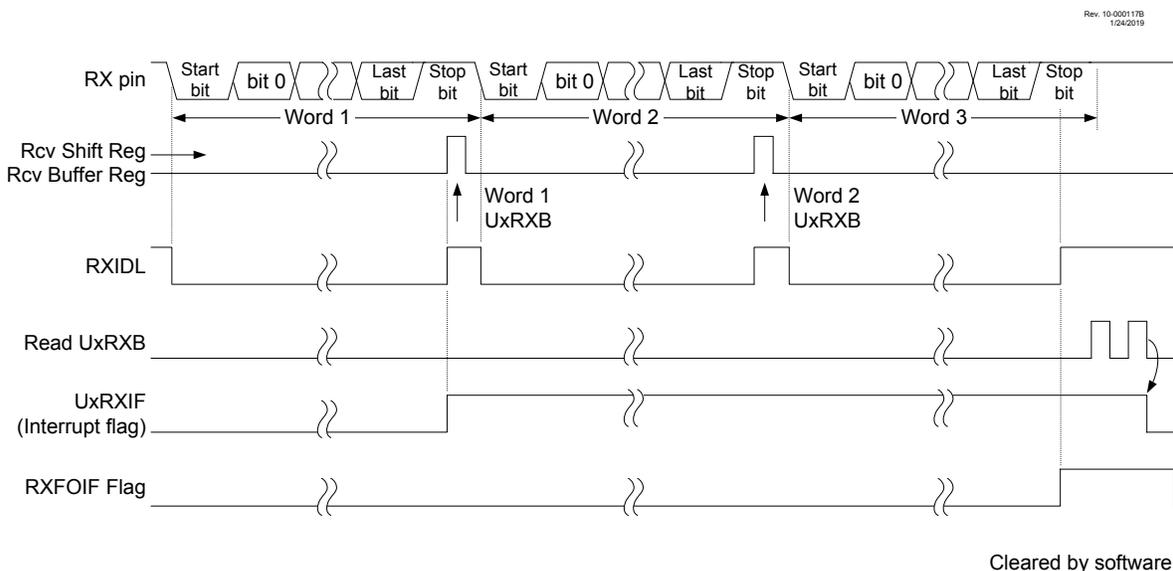
**Note:** This timing diagram shows three bytes appearing on the RX input. The UxRXB is not read before the third word is received, causing the RXFOIF (FIFO overrun) bit to be set. STPMD = 0, STP = 00.
