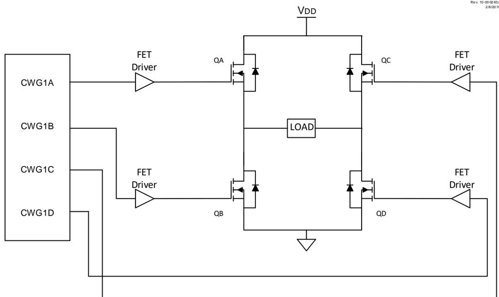
Figure 31-6. Simplified CWG Block Diagram (Forward and Reverse Full Bridge Modes)
