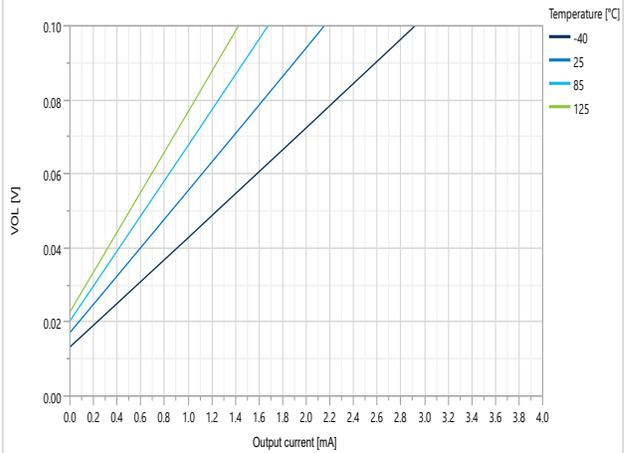
**Figure 49-113.**  $V_{OL}$  at 5V over Temperature and Load Current
