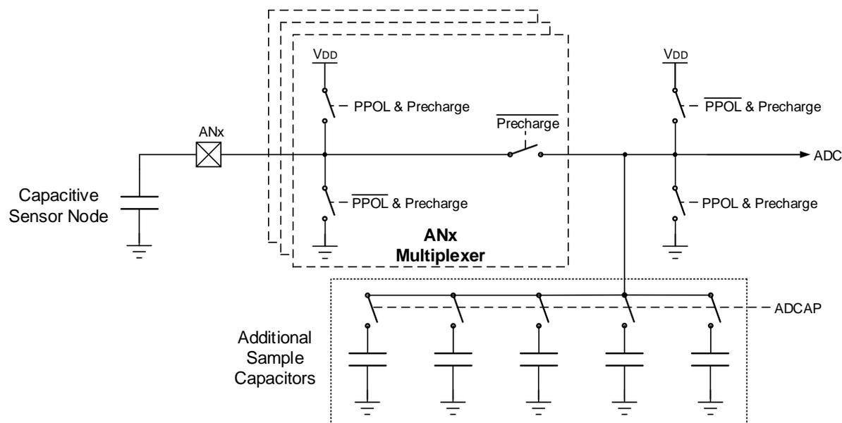
This is an example on how to configure ADC for CVD operation:
