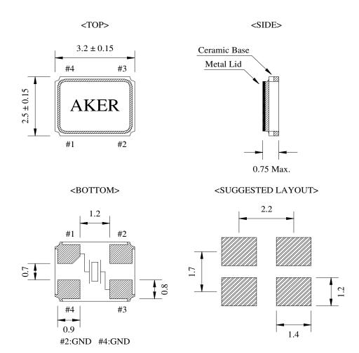
Package is Seam Sealed Ceramic-Metal. Dimensions are millimeters.
