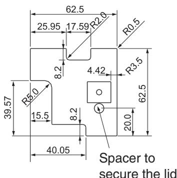
Possibility for integrated battery holder for wireless applications.
