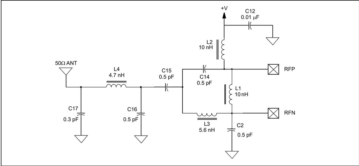
**FIGURE 4-2: BALUN CIRCUIT MEASURED IMPEDANCE**
