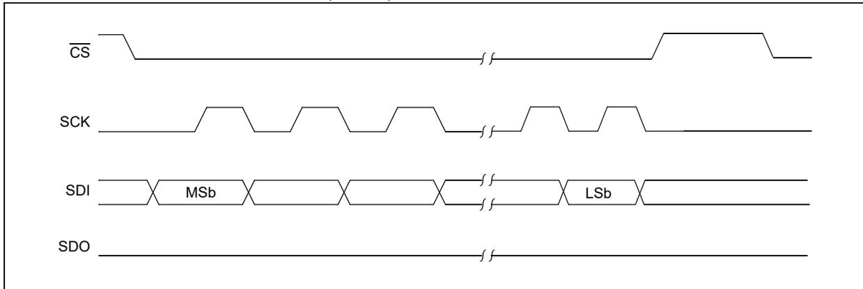
**FIGURE 2-5: SPI PORT READ (OUTPUT) TIMING**
