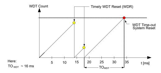
The Normal mode is enabled as long as the Window (WINDOW) bit field in the WDT.CTRLA register is  $0\times0'$ .
