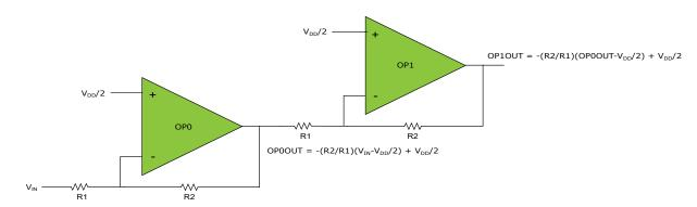
The figure above shows a cascaded inverting PGA constructed from two op amps. The required multiplexer settings are:
