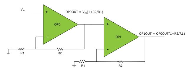
The figure above shows a cascaded non-inverting PGA constructed from two op amps. The following multiplexer settings are required:
