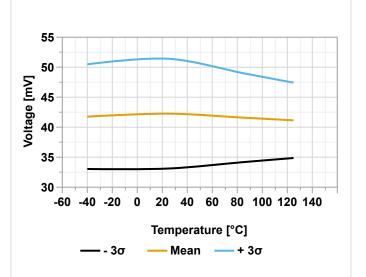
Figure 40-55. BOD Hysteresis vs. Temperature (BODCFG.LVL =
