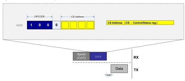
Figure 37-12 shows a typical example of LDCS data transmission. A data byte from the LDCS is transmitted from the UPDI after the guard time is completed.
