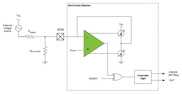
The resistor adds a bias to the ZCD input pin so that the external voltage source must go to zero to pull the pin voltage to the  $Z_{CPINV}$  switching voltage. The pull-up or pull-down value can be determined with the equations shown below.
