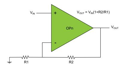
The figure above displays a non-inverting Programmable Gain Amplifier. The required multiplexer settings are as follows:
