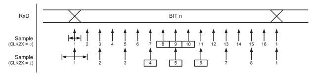
A majority voting technique is, like with clock recovery, used on the three center samples for deciding the logic level of the received bit. The process is repeated for each bit until a complete frame is received.
