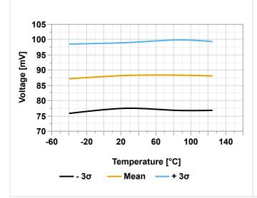
Figure 40-59. VLM Threshold vs. Temperature (VLMCTRL.VLMLVL =  $0 \times 01$ )
