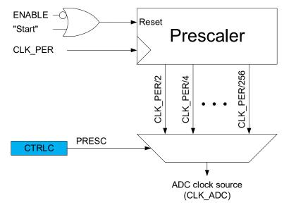
When initiating a conversion by writing a '1' to the Start Conversion (STCONV) bit in the ADCn.COMMAND register or from event, the conversion starts after one CLK\_PER cycle. The prescaler is kept in Reset, as long as there is no ongoing conversion. This assures a fixed delay from the trigger to the actual start of a conversion of maximum two CLK\_PER cycles.
