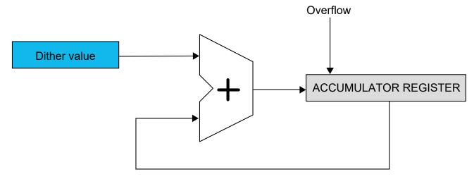
The user can select where in the TCD cycle the dither will be added by writing to the Dither Selection (DITHERSEL) bit field in the Dither Control (TCDn.DITCTRL) register:
