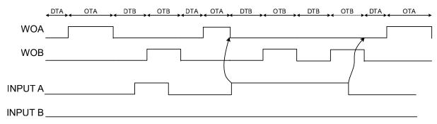
If Input mode 3 is used on input B, an event will only affect if the TCD is in dead-time B or on-time B.
