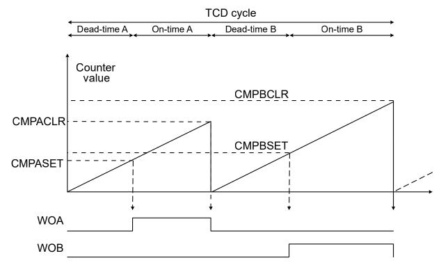
In the figure above, *CMPASET < CMPACLR* and *CMPBSET < CMPBCLR*. This causes the outputs to go high. There are no restrictions on the CMPASET and CMPACLR compared to the CMPBSET and CMPBCLR values.
