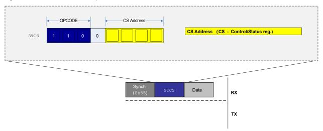
Figure 37-13 shows the data frame transmitted after the SYNCH character and the instruction frames. The STCS instruction byte can immediately be followed by the data byte. There is no response generated from the STCS instruction, as is the case for the ST and STS instructions.
