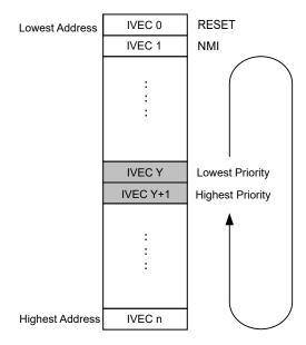
Here, value Y has been written to CPUINT.LVLOPRI so that the interrupt vector Y+1 has the highest priority. Note that, In this case, the priorities will wrap so that the lowest address no longer has the highest priority, not including RESET and NMI, which will always have the highest priority.
