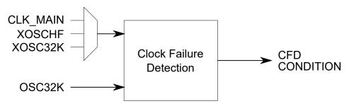
When the CFD feature is enabled, it will monitor the selected source from the Clock Failure Detection Source (CFDSRC) bit field in the Main Clock Control C (CLKCTRL.MCLKCTRLC) register. In sleep, the CFD will only be enabled if the selected source is active.
