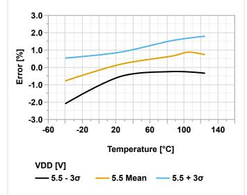
Figure 40-88. ADCOREF Voltage Error vs. Temperature ( $V_{DD} = 3.0V$ ,  $V_{VREF} = 2.5V$ )
