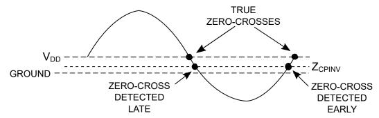
The actual offset time can be determined for sinusoidal waveforms of a known frequency f using the equations shown below.
