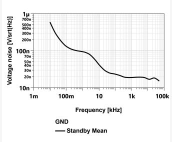
Figure 40-164. Voltage Noise Density for OP2 with IRSEL = 1 and CPU Mode = Standby
