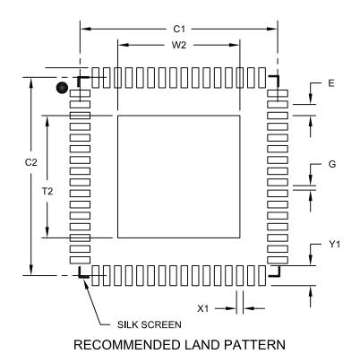
MILLIMETERS Units **Dimension Limits** MIN NOM MAX 0.50 BSC Contact Pitch Ε Optional Center Pad Width W2 5.50 Optional Center Pad Length T2 5.50 Contact Pad Spacing C1 8.90 C2 Contact Pad Spacing 8.90 0.30 Contact Pad Width (X64) X1 Contact Pad Length (X64) Y1 0.85 0.20 Distance Between Pads G
