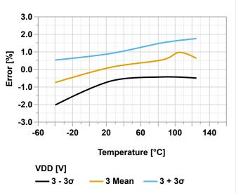
Figure 40-94. ACREF Voltage Error vs. Temperature ( $V_{DD}$  = 5.5V,  $V_{VREF}$  = 2.5V)
