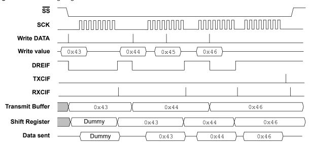
Figure 28-3. SPI Timing Diagram in Buffer Mode with BUFWR in SPIn.CTRLB Written to '0'
