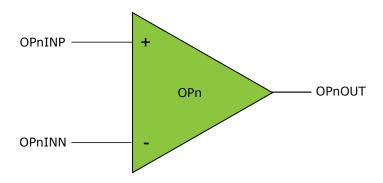
The figure above displays an op amp connected directly to the pins of the device without being connected to any of the internal resistors. This is useful for situations where the user desires to make all connections to other components externally. The multiplexer settings required to achieve this configuration are:
