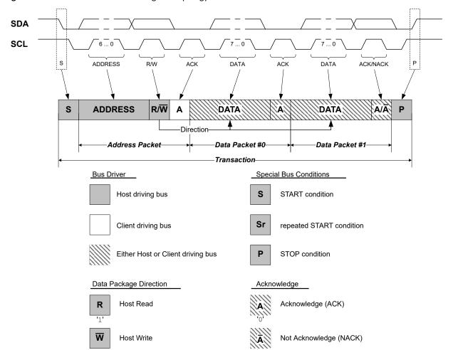
Figure 29-2. Basic TWI Transaction Diagram Topology for a 7-Bit Address Bus
