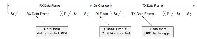
The UPDI guard time is the minimum Idle time that the connected debugger will experience when waiting for data from the UPDI. The maximum Idle time is the same as time-out. When the synchronization time plus the data bus accessing time is longer than the guard time, the Idle time before a transmission will be more than the expected guard time.
