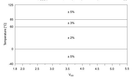
**Note:** The figure is applicable only for  $f_{OSCHF} \ge 4$  MHz.
