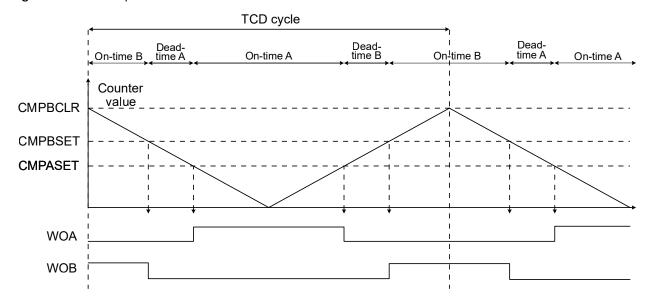
When starting the TCD in Dual Slope mode, the TCD counter starts at the CMPBCLR value and counts down. In the first cycle, the WOB will not be set until the TCD counter matches the CMPBSET value when counting up.
