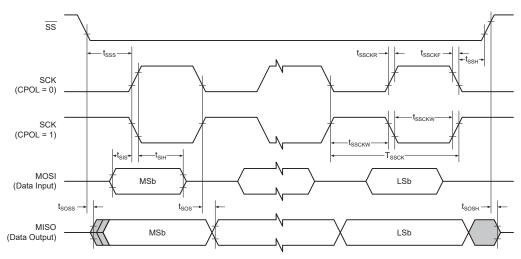
Table 39-21. SPI - Timing Specifications in Client Mode
