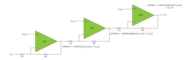
The figure above shows a cascaded inverting PGA constructed from three op amps. The required multiplexer settings are:
