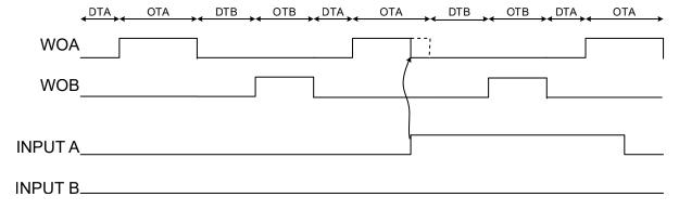
If Input mode 9 is used on input B and a positive edge on the input event occurs while in on-time B, the output will be OFF for the rest of the on-time.
