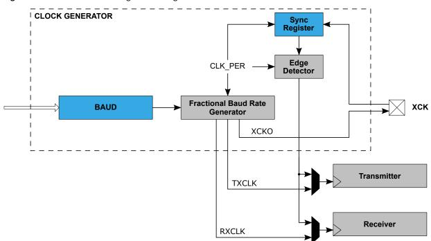
Figure 27-3. Clock Generation Logic Block Diagram
