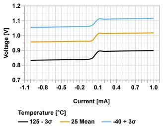
Figure 40-194. Zero-Cross Detector Trip Voltage vs. V<sub>DD</sub>
