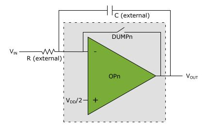
The figure above shows how an op amp can be configured as an integrator. An external capacitor and external resistor are required. The DUMPn event closes a switch to discharge the capacitor and reset the integrator. The multiplexer settings required are:
