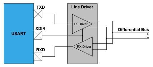
The XDIR pin goes high one baud clock cycle in advance of data being shifted out to allow some guard time to enable the external line driver. The XDIR pin will remain high for the complete frame, including Stop bit(s).
