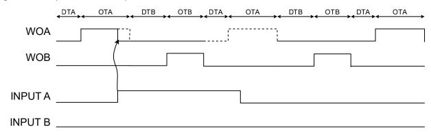
If Input mode 10 is used on input B and an input event occurs, the WOB will be OFF as long as the event lasts. If released during an on-time, it will be OFF for the rest of the on-time.
