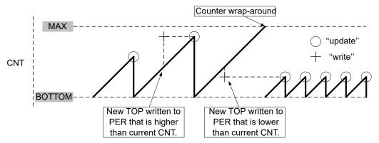
A counter wrap-around can occur in any mode of operation when counting up without buffering, as the TCAn.CNT and TCAn.PER registers are continuously compared. If writing a new TOP value to TCAn.PER lower than the current TCAn.CNT, the counter will wrap first before a compare match occurs.
