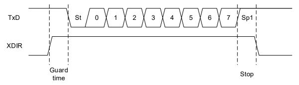
RS-485 mode is compatible with One-Wire mode. One-Wire mode enables an internal connection between the TXD pin and the USART receiver, making the TXD pin a combined TxD/RxD line. The RXD pin will be disconnected from the USART receiver and may be controlled by a different peripheral. An example of such a circuit is shown in the figure below.
