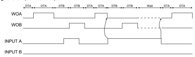
If Input mode 2 is used on input B, an event will only affect if the TCD is in dead-time B or on-time B, and it will affect only the WOB output.
