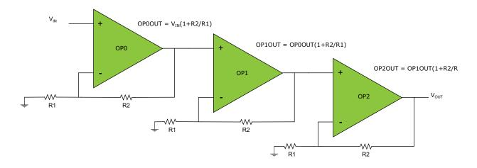
The figure above shows a cascaded non-inverting PGA constructed from three op amps. The following multiplexer settings are required:
