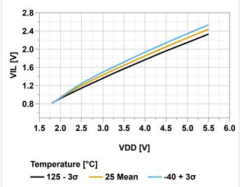
Figure 40-69. Input Pin with I<sup>2</sup>C Trigger - Maximum V<sub>IL</sub> vs. V<sub>DD</sub> Figure 40-70. Input Pin with I<sup>2</sup>C Trigger - Minimum V<sub>IH</sub> vs. V<sub>DD</sub>
