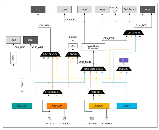
The clock system consists of the main clock and clocks derived from the main clock, as well as several asynchronous clocks:
