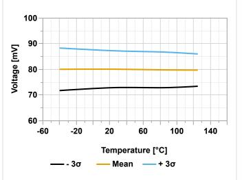
Figure 40-58. BOD Hysteresis vs. Temperature (BODCFG.LVL =  $0 \times 03)$
