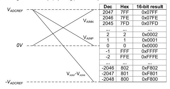
If a single-ended analog input is above the ADC voltage reference level, the 12-bit ADC result will be 0xFFF (decimal 4095). Likewise, if it is below 0V, the ADC result will be 0x000.
