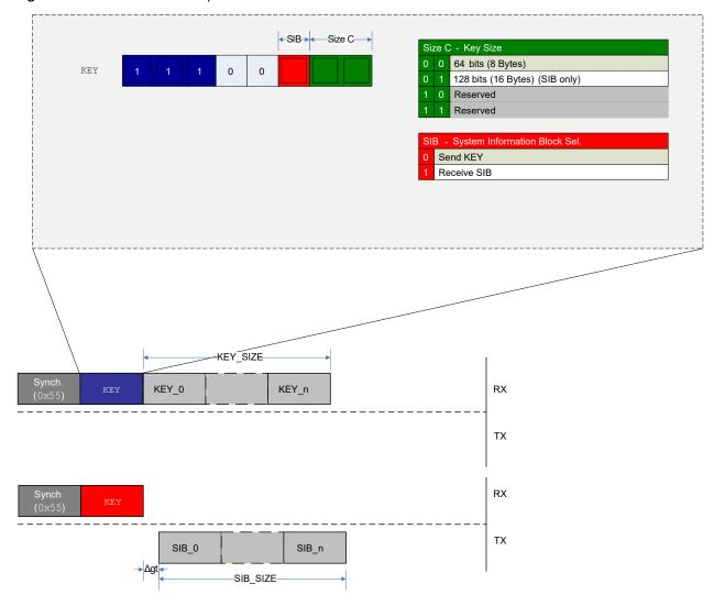
Figure 37-16 shows the transmission of a key and the reception of a SIB. In both cases, the Size C (SIZE\_C) field in the operand determines the number of frames being sent or received. There is no response after sending a KEY to the UPDI. When requesting the SIB, data will be transmitted from the UPDI according to the current guard time setting.
