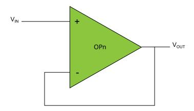
The figure above displays a voltage follower, also known as a unity-gain buffer. The non-inverting (+) input is connected to a pin, and the output is connected to the inverting (-) input. The multiplexer settings required for this configuration are:
