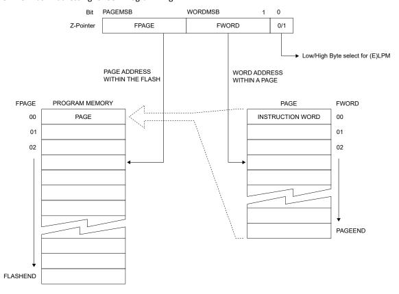
The Flash is word-accessed and organized in pages, so the Address Pointer can be treated as having two sections, as shown in the figure above. The word address in the page (FWORD) is held by the Least Significant bits (LSbs) in the Address Pointer, while the Most Significant bits (MSbs) in the Address Pointer hold the Flash page address (FPAGE). Together, FWORD and FPAGE hold an absolute address to a word in the Flash.
