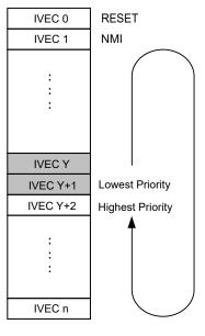
The round robin scheduling for LVL0 interrupt requests is enabled by writing a '1' to the Round Robin Priority Enable (LVL0RR) bit in the Control A (CPUINT.CTRLA) register.
