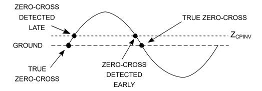
When the waveform is referenced to  $V_{DD}$ , as shown in the figure below, the zero-cross is detected too late as the waveform falls and too early as the waveform rises.
