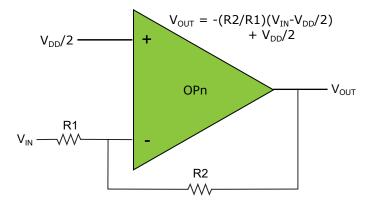
The figure above shows the inverting PGA configuration. The multiplexer settings required are:
