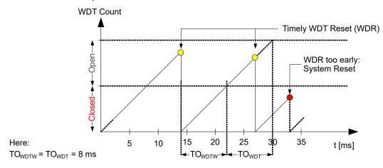
The Window mode is enabled by writing a non-zero value to the WINDOW bit field in the Control A (WDT.CTRLA) register and disabled by writing it to 0x0.
