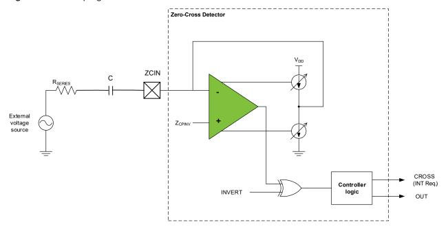
The phase shift resulting from the capacitor will cause the ZCD output to switch in advance of the actual zero-crossing event. The phase shift will be the same for both rising and falling zero-crossings, which can be compensated for by either delaying the CPU response to the ZCD switch by a timer or other means or selecting a capacitor value large enough that the phase shift is negligible.
