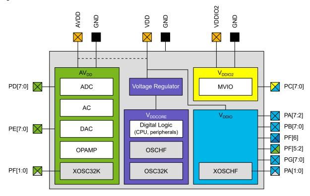
**Note:** For the AVR® DBFamily of devices, AVDD is internally connected to VDD (not separate power domains).
