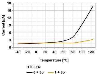
Figure 40-17. Typical +3 $\sigma$  Power-Down Power Consumption vs. Temperature (V<sub>DD</sub> = 5.5V)
