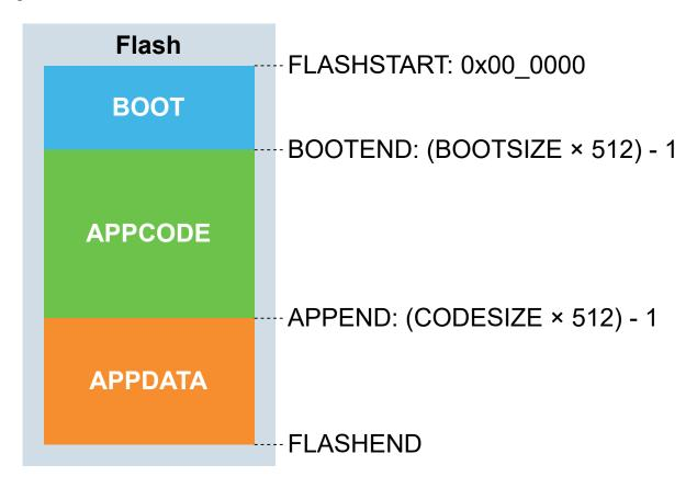
If FUSE.BOOTSIZE is written to '0' Flash is regarded as the BOOT section. If FUSE.CODESIZE is written to '0' and FUSE.BOOTSIZE > 0, the APPCODE section runs from BOOTEND to the end of Flash (no APPDATA section).
