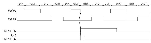
If Input mode 8 is used on input B and a positive edge on the input event occurs while in on-time B, the TCD counter jumps to dead-time A.
