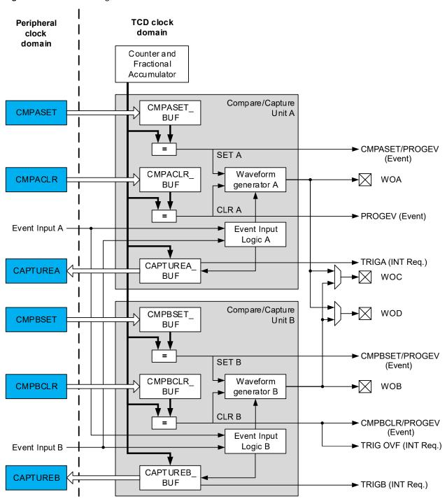
The TCD core is asynchronous to the peripheral clock. The timer/counter consists of two compare/capture units, each with a separate waveform output. There are also two extra waveform outputs, which can be equal to the output from one of the units. For each compare/capture unit, there is a pair of compare registers which is stored in the respective peripheral (TCDn.CMPASET, TCDn.CMPBCLR, TCDn.CMPBSET, TCDn.CMPBCLR) registers.
