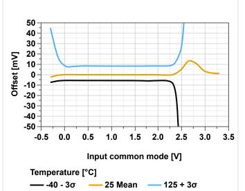
Figure 40-178. Offset Over Temperature with  $V_{DD} = 1.8V$ 7.5 5 Offset [mV] 2.5 0 -2.5 -5 -7.5 0 50 100 -50 Temperature [°C] VDD [V] <del>--</del> 1.8 - 3σ 1.8 Mean
