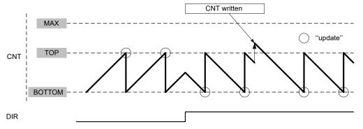
It is possible to change the counter value in the Counter (TCAn.CNT) register when the counter is running. The write access to TCAn.CNT register has higher priority than count, clear or reload, and will be immediate. The direction of the counter can also be changed during ordinary operation by writing to the Direction (DIR) bit in the Control E (TCAn.CTRLE) register.
