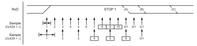
A new high-to-low transition indicating the Start bit of a new frame can come right after the last of the bits used for majority voting. For Normal-Speed mode, the first low-level sample can be at the point marked (A) in the figure above. For Double-Speed mode, the first low level must be delayed to point (B), being the first sample after the majority vote samples. Point (C) marks a Stop bit of full length at the nominal baud rate.
