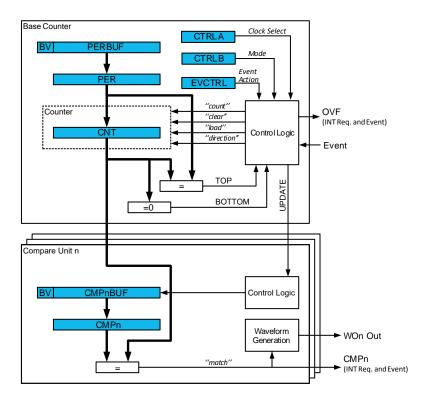
The Counter (TCAn.CNT) register, Period and Compare (TCAn.PER and TCAn.CMPn) registers, and their corresponding buffer registers (TCAn.PERBUF and TCAn.CMPnBUF) are 16-bit registers. All buffer registers have a Buffer Valid (BV) flag indicating when the buffer contains a new value.
