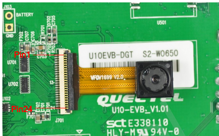
Figure 37: Installation of the camera module.
