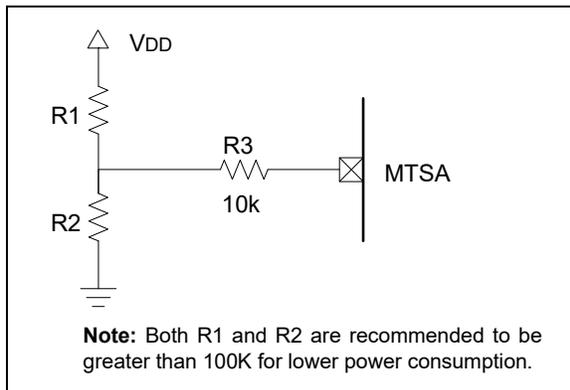
**FIGURE 3-2: HARDWARE SENSITIVITY ADJUST USING POTENTIOMETER**
