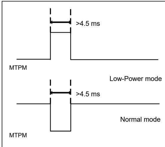
**Note:** In non-detected state, because the device goes to Sleep for a certain time, the Reset pulse duration should be 4.5 ms plus the Sleep time.
