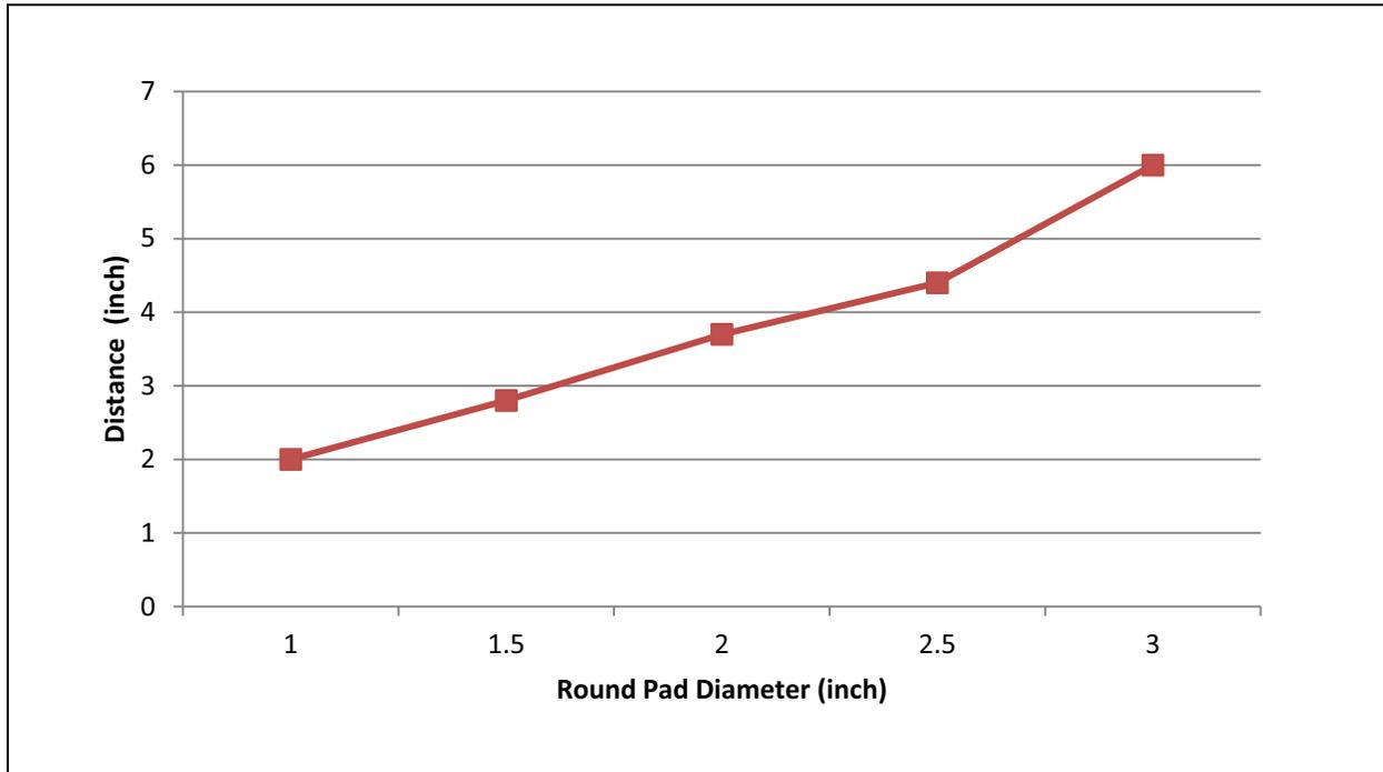
**Note:** The tested sensors are round solid pads on FR4 PCB. No ground plane was near the sensor, as this would give the maximum detection distance.
