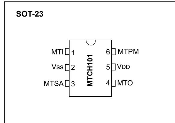
**TABLE 1: 6-PIN SOT-23 PINOUT DESCRIPTION**
