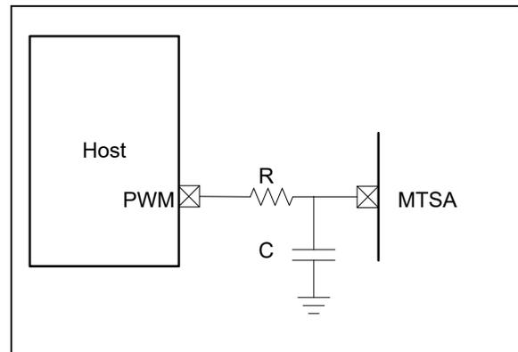
**Note 1:** Application Note AN538, "Using PWM to Generate Analog Output" has details about how to choose appropriate R and C values.
