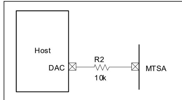
**FIGURE 3-4: SENSITIVITY CONTROLLED BY HOST USING PWM**
