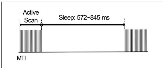
**Note:** If the device makes a proximity or touch detection, it will automatically perform active scans continually. Once the device releases from its proximity-detected state, it will return to the power mode set by the MTPM pin.
