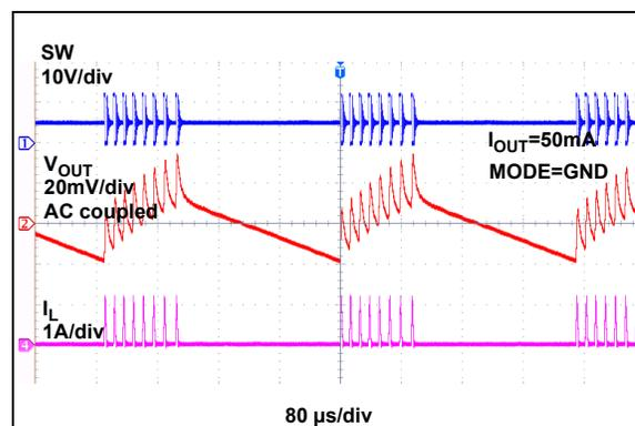
**FIGURE 2-35:** Switching Waveform ( $I_{OUT} = 0.05A$ ) - HLL.
