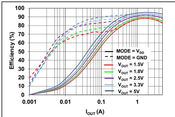
**FIGURE 2-2:** Efficiency vs. Output Current ( $V_{IN} = 12V$ ).
