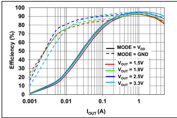
**FIGURE 2-1:** Efficiency vs. Output Current ( $V_{IN} = 5V$ ).
