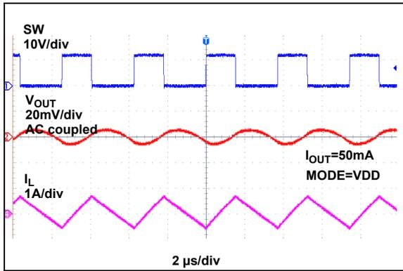
**FIGURE 2-37:** Switching Waveform ( $I_{OUT} = 0.05A$ ) - CCM.
