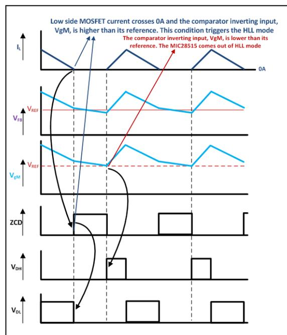
**FIGURE 4-3:** MIC28515 Control Loop Timing (HLL Mode).
