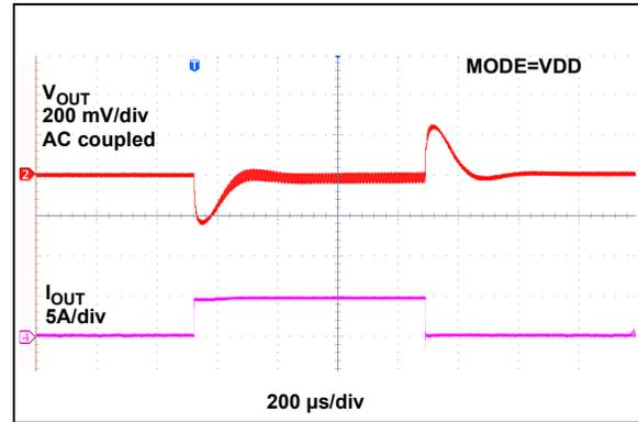
**FIGURE 2-47:** Load Transient Response (0 to 5A) - CCM.
