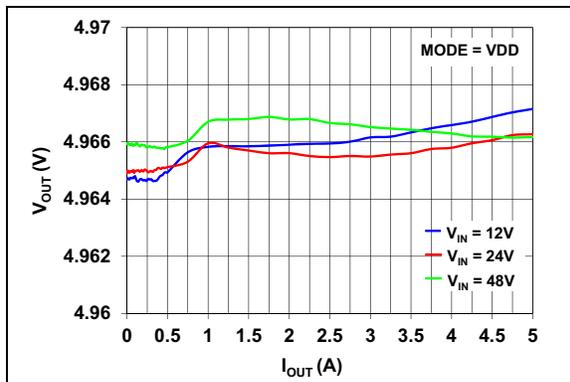
**FIGURE 2-8:** Output Voltage vs. Output Current ( $V_{OUT} = 5V$ ).
