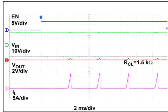
**FIGURE 2-40:** Enable into Short-Circuit.
