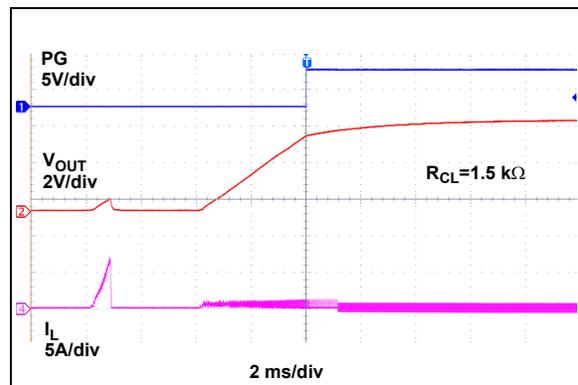
**FIGURE 2-42:** Recovery from Short-Circuit.
