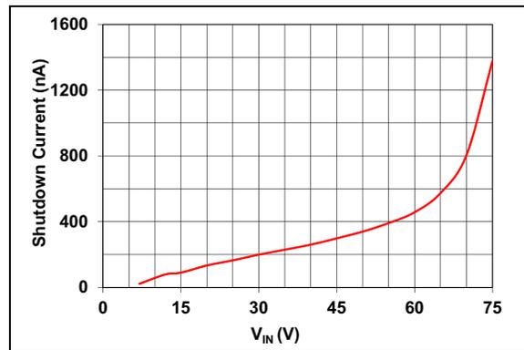
**FIGURE 2-17:**  $V_{IN}$  Shutdown Current vs. Input Voltage.
