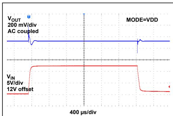
**FIGURE 2-49:** Line Transient Response (12V to 24V).
