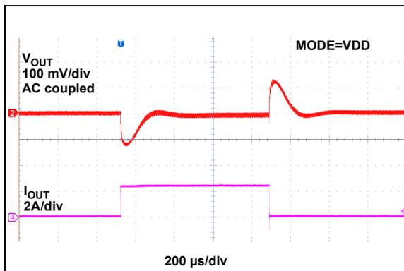
**FIGURE 2-45:** Load Transient Response (0 to 2.5A).
