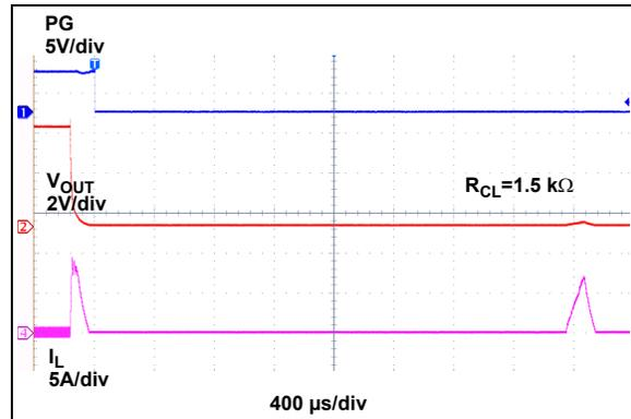
**FIGURE 2-41:** Behavior when Entering Short-Circuit.
