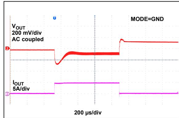
**FIGURE 2-46:** Load Transient Response (0 to 5A) - HLL.
