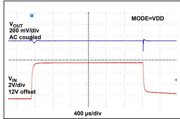
**FIGURE 2-48:** Line Transient Response (12V to 18V).
