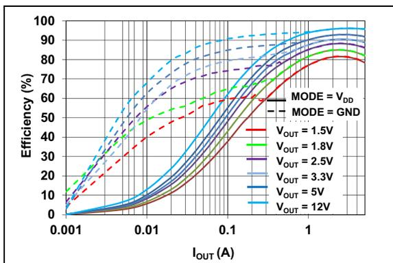
**FIGURE 2-3:** Efficiency vs. Output Current ( $V_{IN} = 24V$ ).
