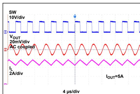
**FIGURE 2-36:** Switching Waveform ( $I_{OUT} = 5A$ ).
