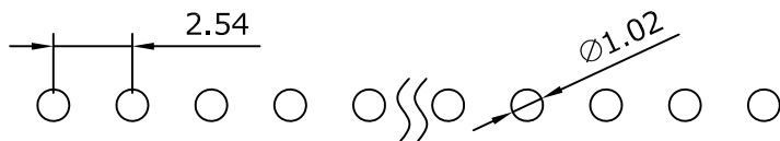
Recommended PCB Layout (PCB TOLERANCE ±0.05)
