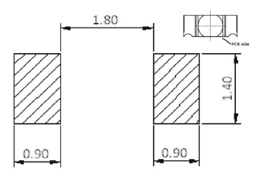
Metalization layer is thicker than the solder resist layer. Recommended solder thickness: 120 - 150  $\mu m$ .
