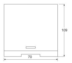
A standard plugable terminal (like Phoenix or any other connector) is mounted with the other components to the PCB.The side parts and and front are screwed to the PCB and slid into the box. The unit is ready. The wire part is then just plugged in.
