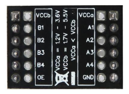
The signals at the inputs/outputs A1-A4 are shifted to the respective voltage level (VCCa  $\rightarrow$  A1-A4 | VCCb  $\rightarrow$  B1-B4)
