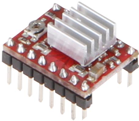
After the jumpers are set, the stepper motor drivers have to be plugged into the black slots which are directly at the jumper slots. Make sure that the stepper motor driver are rightfully plugged in. You can gather the information from the following picture on how to plug in the motor drivers correctly.
