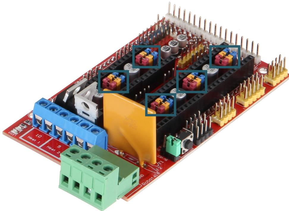
The different jumper slots are shown in the picture above and in the schematic drawing before. The various step configurations are displayed in the following chart.
