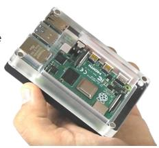
Now stick the enclosed heatsinks onto the Raspberry Pi.
