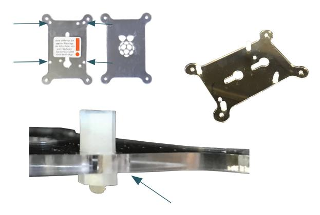
Now you can apply the Raspberry Pi on the spacers and screw it tight with four synthetic screws.
