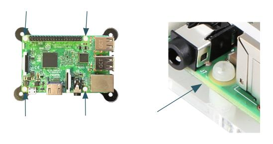
First of all, screw together the base plate (plate with wall mount) and the spacers with threads. You should use the spacers with threads that you can add the next plate on top of the other.
