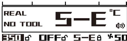
Channel 1 is selected. Sensor failure or no holder available
