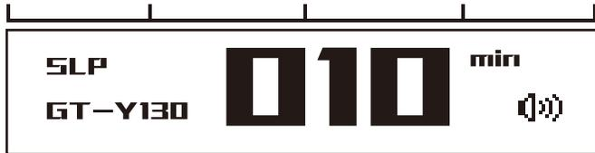
SLP sleep setting dialog (10minutes sleeping duration in the above figure. If the soldering station is not used within 10 minutes, the electrical soldering station will automatically enter into sleeping state.)
