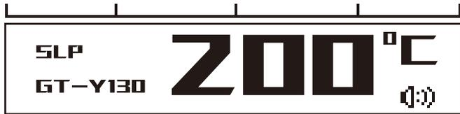
SLP sleeping status indication window (sleeping temperature drops to 200°C when the setting value is higher than 200°C).
