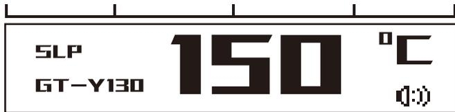
SLP sleeping status indication window (sleeping temperature keep to setting value when the setting value is less than 200°C).
