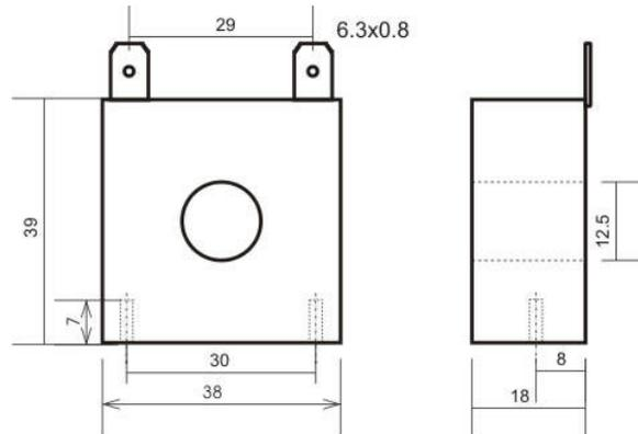
ANG company produces high quality current transformers with guaranteed precision. The following types 50A/0.05A, 100A/0.05A, 150A/0.05A and 200A/0.05A are available. Custom types are also available.
