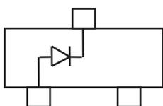
**350mW 100Volt Switching Diode**
