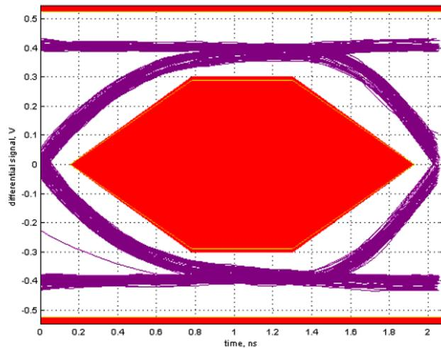
Figure 10.2 USB-IF High-speed Eye Diagram (with data switch)
