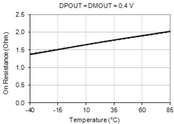
**Figure 10.10 Power Switch On Resistance vs. Temp**
