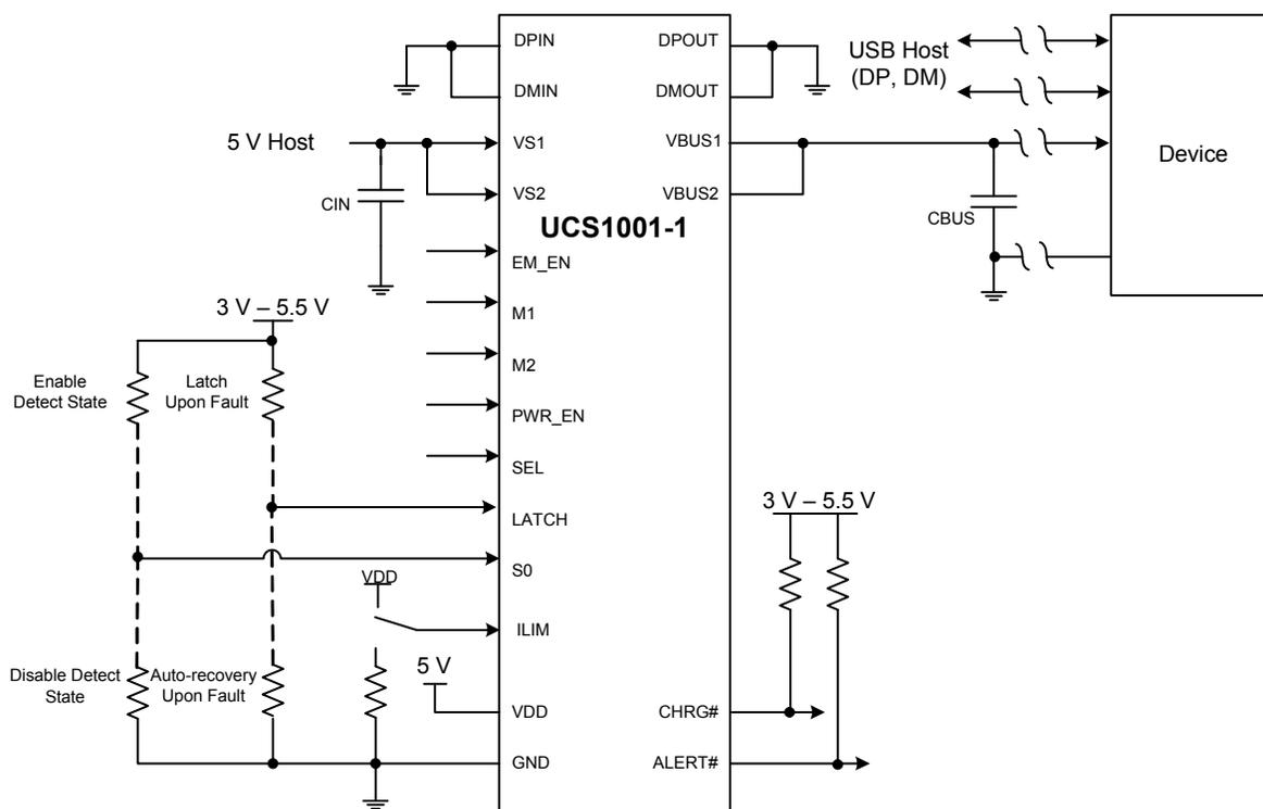
Figure 4.1 UCS1001-1 System Configuration (No Charger Emulation)
