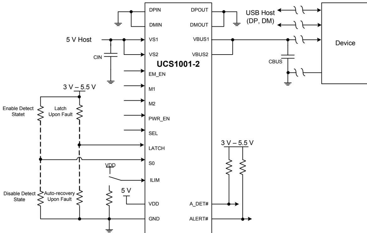
**Figure 4.2 UCS1001-2 System Configuration (No Charger Emulation)**
