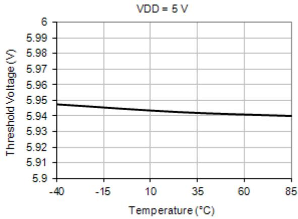
**Figure 10.14 VS Under Voltage Threshold vs. Temp**
