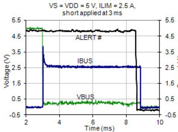
Figure 10.4 Power Up Into A Short
