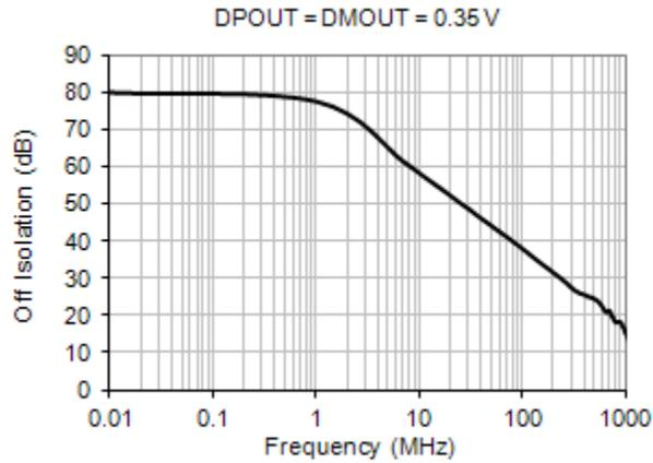
**Figure 10.8 Data Switch Bandwidth vs. Frequency**
