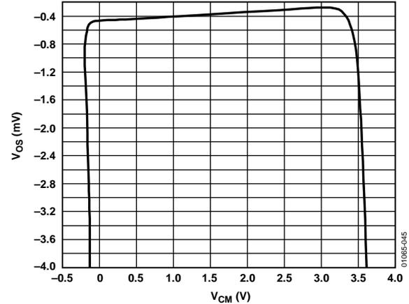
Figure 45.  $V_{os}$  vs. Common-Mode Voltage,  $V_s = 5$  V
