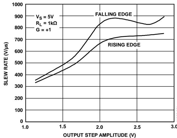
Figure 24. Slew Rate vs. Output Step Amplitude
