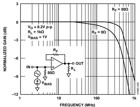
Figure 5. Small Signal Response,  $R_F = 0 \Omega$ ,  $50 \Omega$
