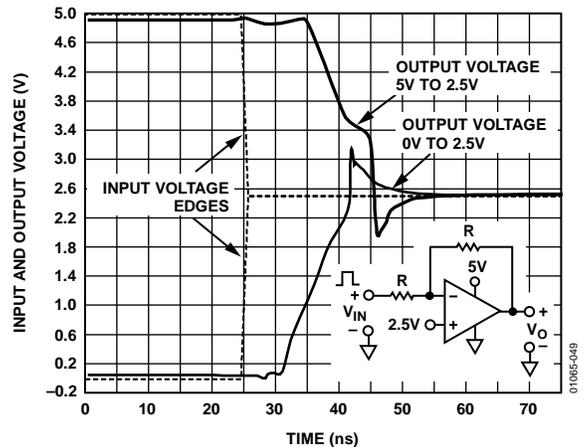
Figure 49. Overload Recovery,  $G = -1$ ,  $V_S = 5\text{ V}$
