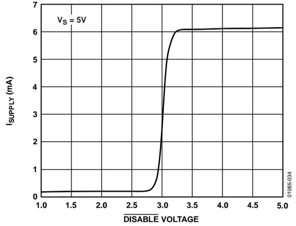
Figure 34. AD8063  $\overline{\text{DISABLE}}$  Voltage vs. Supply Current
