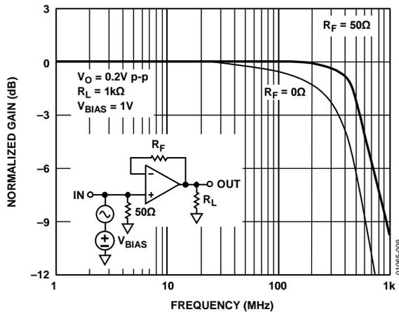
Figure 9. Small Signal Response,  $R_F = 0\Omega, 50\Omega$
