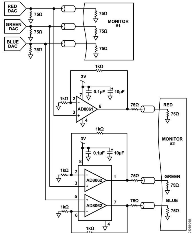
Figure 55. RGB Cable Driver Using AD8061 and AD8062
