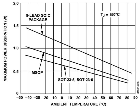
Figure 6. Maximum Power Dissipation vs. Temperature for AD8061/AD8062/AD8063
