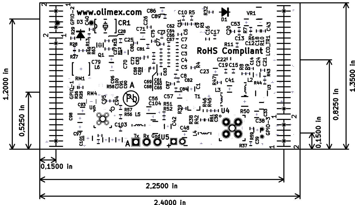
Board dimensions are: 2.4 inch (60.96 mm) x 1.2 inch (30.48 mm).
