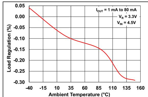
**FIGURE 2-6:** Load Regulation vs. Ambient Temperature ( $V_R = 3.3\text{V}$ ).
