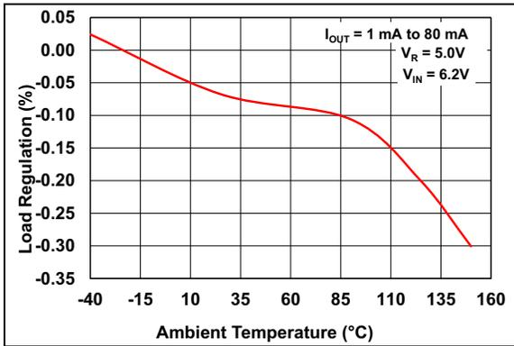
**FIGURE 2-7:** Load Regulation vs. Ambient Temperature ( $V_R = 5.0\text{V}$ ).
