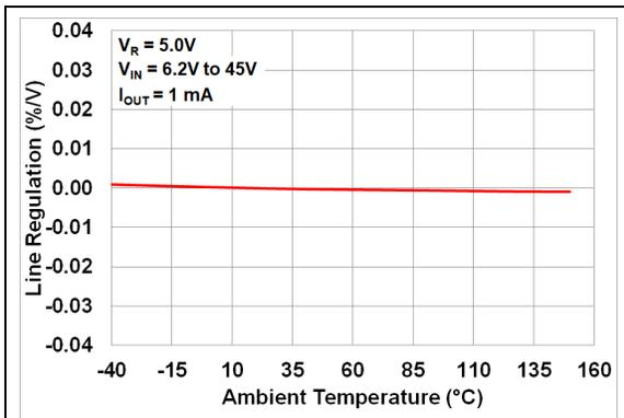
**FIGURE 2-9:** Line Regulation vs. Ambient Temperature ( $V_R = 5.0\text{V}$ ).
