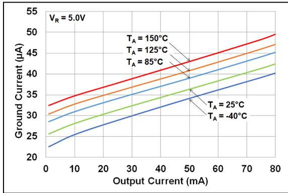
**FIGURE 2-13:** Ground Current vs. Output Current ( $V_R = 5.0\text{V}$ ).
