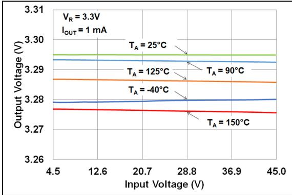
**FIGURE 2-1:** Output Voltage vs. Input Voltage ( $V_R = 3.3\text{V}$ ).
