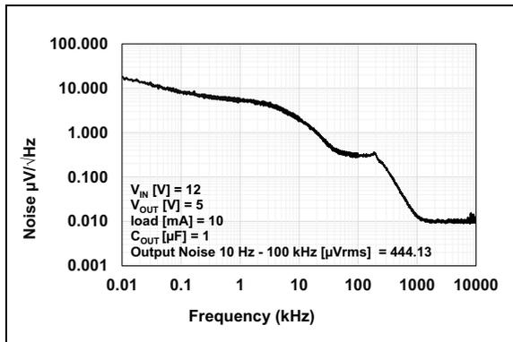
**FIGURE 2-15:** Noise vs. Frequency ( $V_R = 5.0\text{V}$ ).
