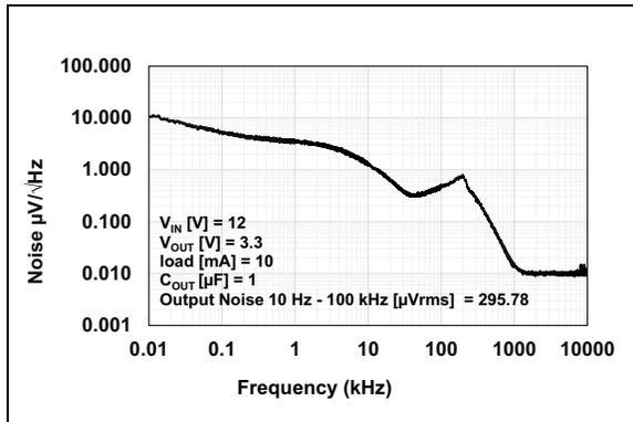
**FIGURE 2-14:** Noise vs. Frequency ( $V_R = 3.3\text{V}$ ).
