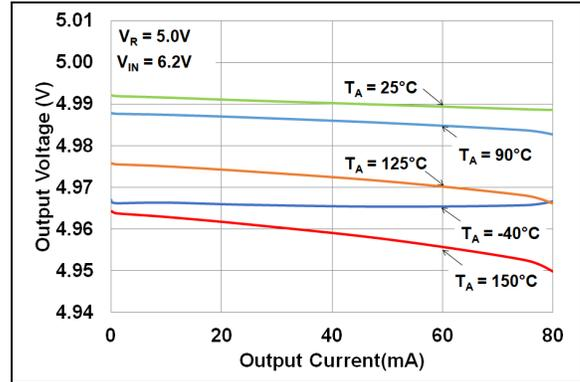
**FIGURE 2-4:** Output Voltage vs. Output Current ( $V_R = 5.0\text{V}$ ).
