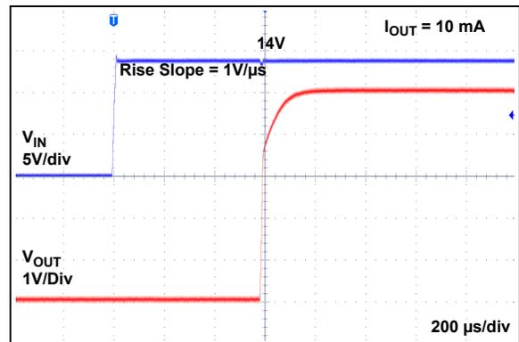
**FIGURE 2-23:** Start-up ( $V_R = 5.0\text{V}$ ).
