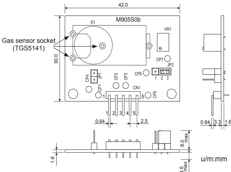
\* The sensor is to be put in the sensor socket as shown in the above photo.
