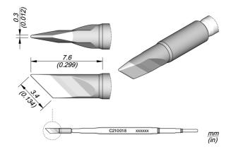
C210 cartridges are appropriate for precision soldering jobs with medium power requirements.
