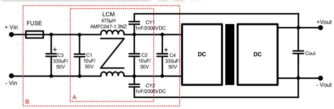
Notes:Part A for EMI filtering and Part B is used for EMS test.
