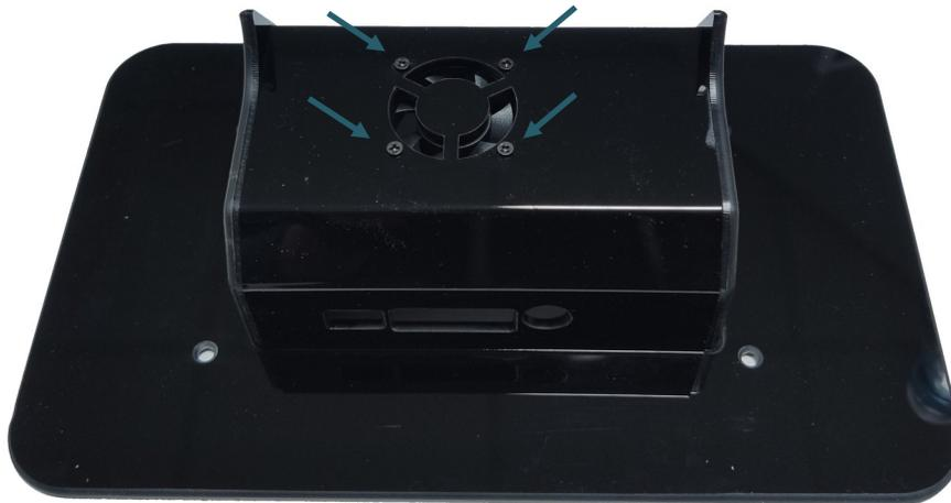
6. Connect the fan to the Raspberry Pi.
