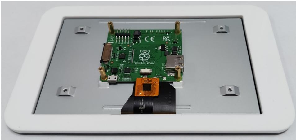
2. Now connect the cables which are in the scope of delivery of the display, to the display board. Make sure that the display cable is aligned correctly.
