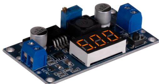
This is a voltage converter based on the DC-DC module LM2596S. The voltage can be adjusted by the potentiometer with an accuracy of  $\pm 0.1$  V (DC). The integrated segment display can additionally be switched between the input and the output voltage via the button.
