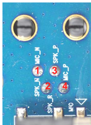
Figure 15: Pin Assignments of Handset Interface J503
