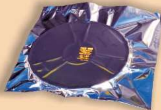
MBB with Recommended Light Air Evacuation
