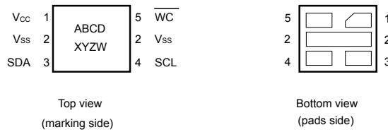
Figure 3. UDFPN5 (DFN5) package connections
