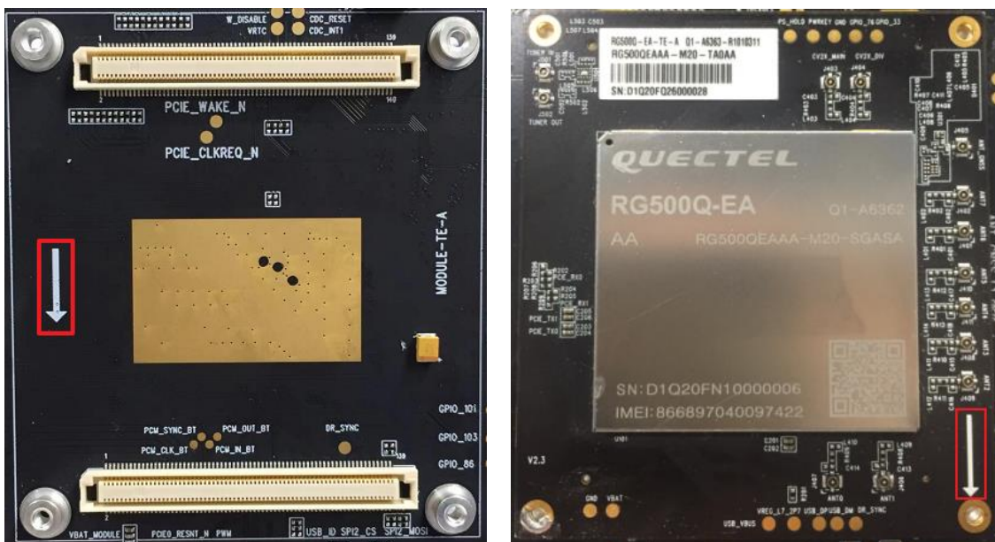
Figure 7: Connection Between the Module TE-A and the EVB
