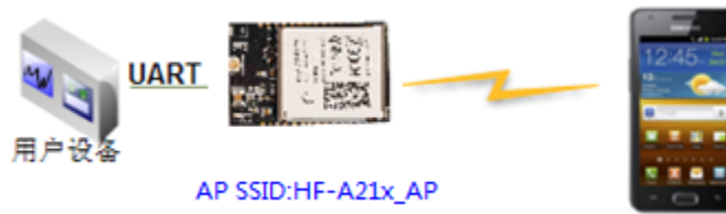
Figure 40. Wireless Control Application
