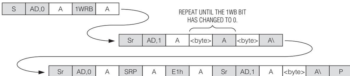
Poll the Status Register until the 1WB bit has changed from 1 to 0. Then set the read pointer to the Read Data Register (code E1h) and access the device again to read the data byte that was obtained from the 1-Wire line.
