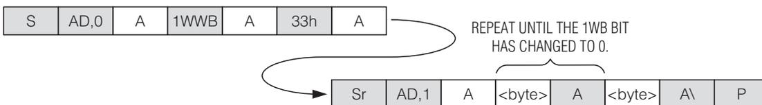
When 1WB has changed from 1 to 0, the 1-Wire Write Byte command is completed.
