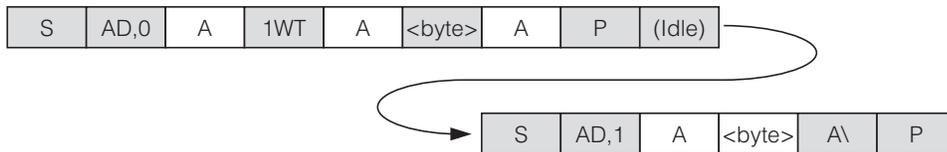
The idle time is needed for the 1-Wire function to complete. Then access the device in read mode to get the result from the 1-Wire Triplet command.
