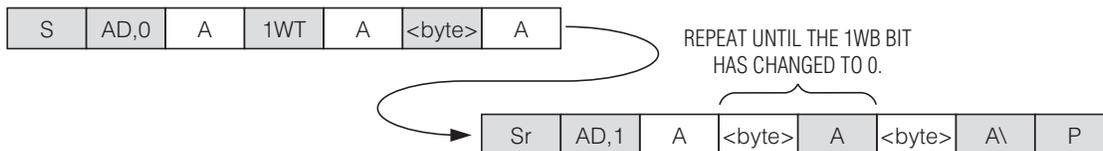
When 1WB has changed from 1 to 0, the Status Register holds the valid result of the 1-Wire Triplet command.
