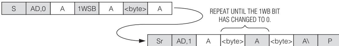
When 1WB has changed from 1 to 0, the Status Register holds the valid result of the 1-Wire Single Bit command.
