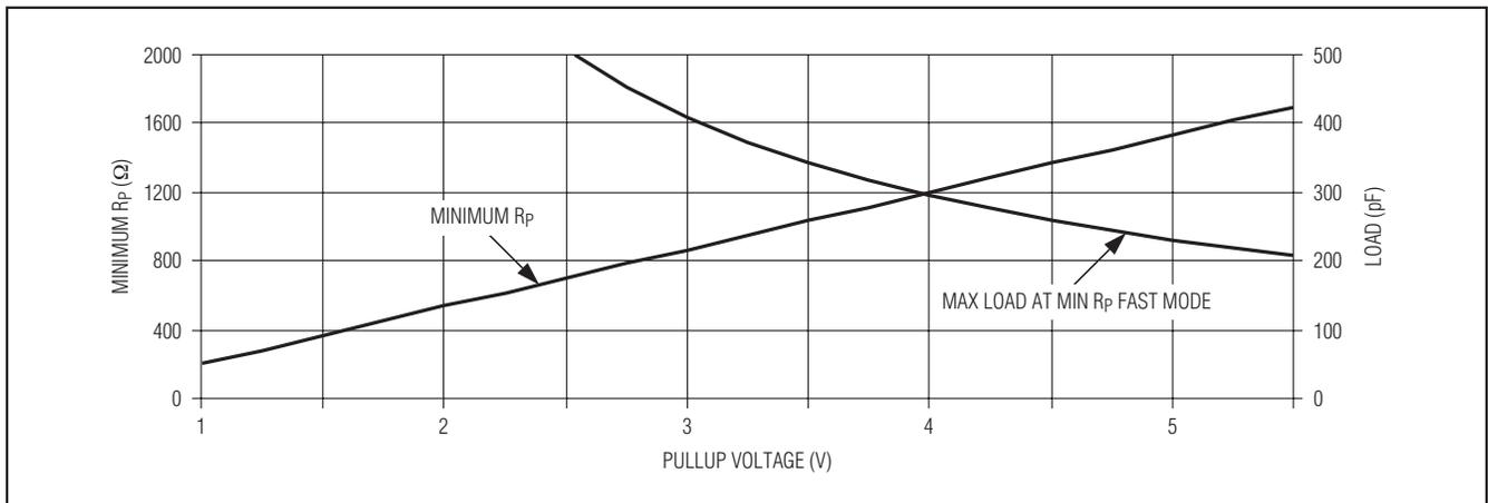
Figure 11. I<sup>2</sup>C Fast Mode Pullup Resistor Selection Chart
