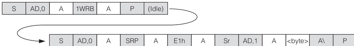
The idle time is needed for the 1-Wire function to complete. Then set the read pointer to the Read Data Register (code E1h) and access the device again to read the data byte that was obtained from the 1-Wire line.
