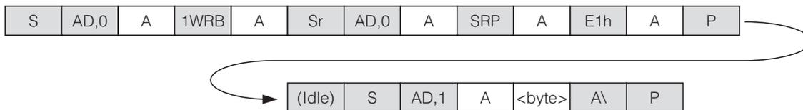
The read pointer is set to the Read Data Register (code E1h) while the 1-Wire Read Byte command is still in progress. Then, after the 1-Wire function is completed, the device is accessed to read the data byte that was obtained from the 1-Wire line.
