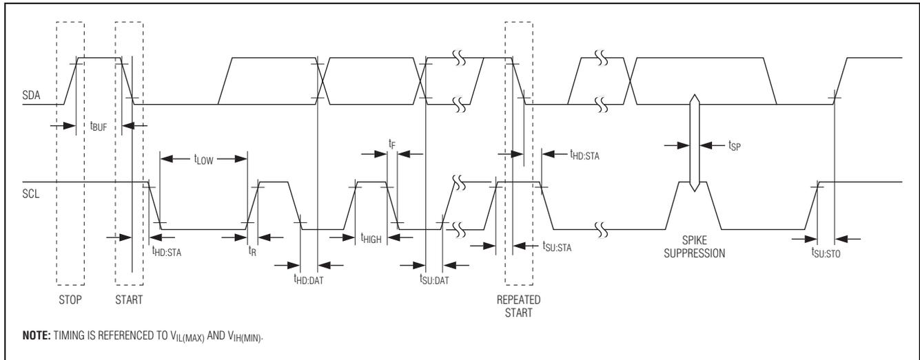
Figure 9. I<sup>2</sup>C Timing Diagram
