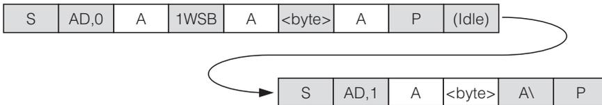
The idle time is needed for the 1-Wire function to complete. Then access the device in read mode to get the result from the 1-Wire Single Bit command.
