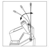
The cable collector is flexible. It accompanies and adapts to the movements during the soldering process.
