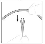
Insert the cable into the clip and then insert into the cable collector. Do not leave the cable longer than necessary to reach the work area freely.
