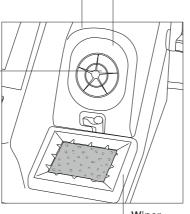
If the tip is very dirty, JBC recommends first cleaning it with the wiper to remove excess solder.
