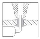
Place the tip with the component terminal in the hole.
