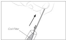
Remove the coil filter, check the filter and replace it if it is dirty or damaged.
