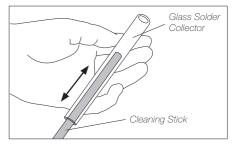
Clean the inside of the glass solder collector with the cleaning stick.
