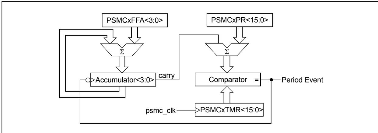
The FFA function is only available when using one of the two Fixed Duty Cycle modes of operation. In fixed duty cycle operation each PWM period is comprised of two period events. That is why the PWM periods in Table 24-3 example calculations are multiplied by 2 as opposed to the normal period calculations for normal mode operation.
