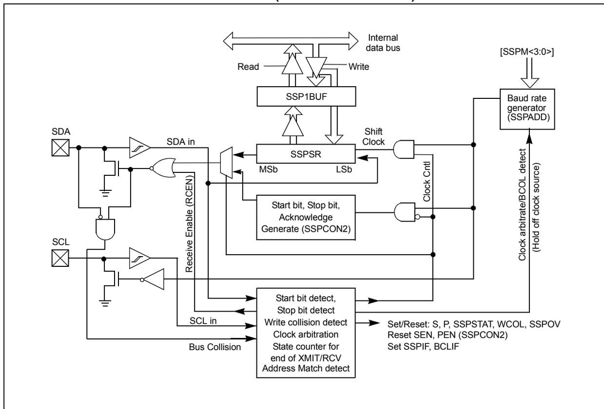
**FIGURE 26-3: MSSP BLOCK DIAGRAM (I<sup>2</sup>C™ SLAVE MODE)**
