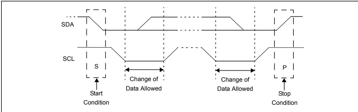
**FIGURE 26-13: I<sup>2</sup>C RESTART CONDITION**
