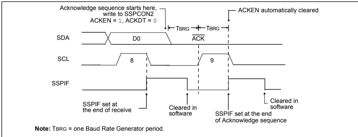
**FIGURE 26-31: STOP CONDITION RECEIVE OR TRANSMIT MODE**
