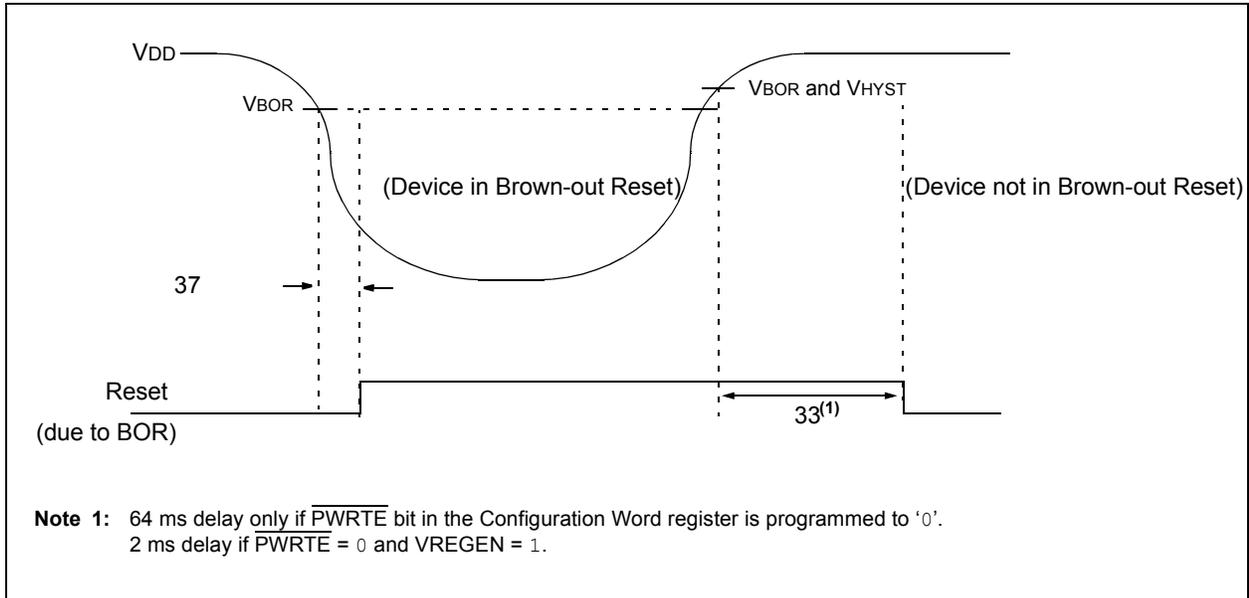
**TABLE 30-5: RESET, WATCHDOG TIMER, OSCILLATOR START-UP TIMER, POWER-UP TIMER AND BROWN-OUT RESET PARAMETERS**
