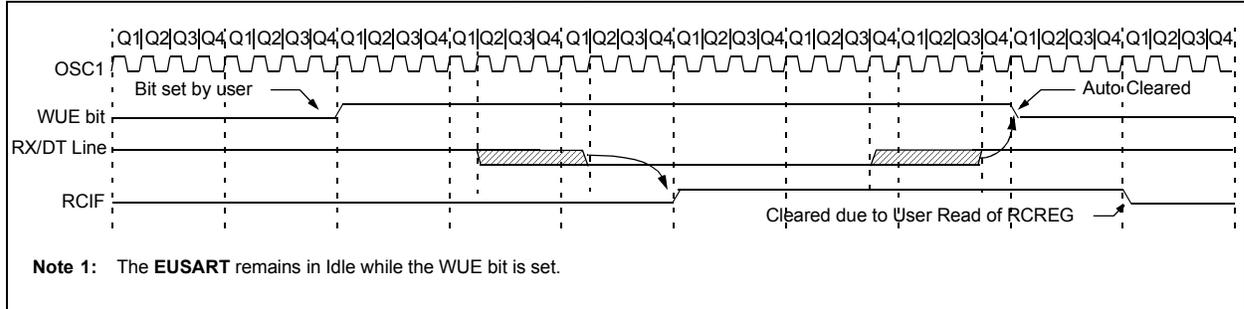
**FIGURE 27-8: AUTO-WAKE-UP BIT (WUE) TIMINGS DURING SLEEP**
