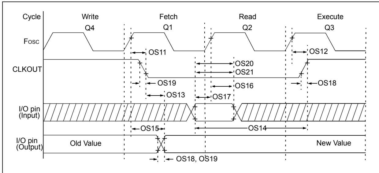
**TABLE 30-4: CLKOUT AND I/O TIMING PARAMETERS**
