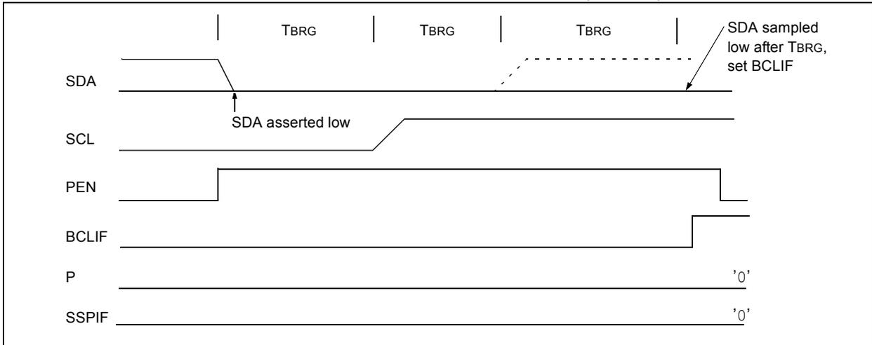
**FIGURE 26-39: BUS COLLISION DURING A STOP CONDITION (CASE 2)**
