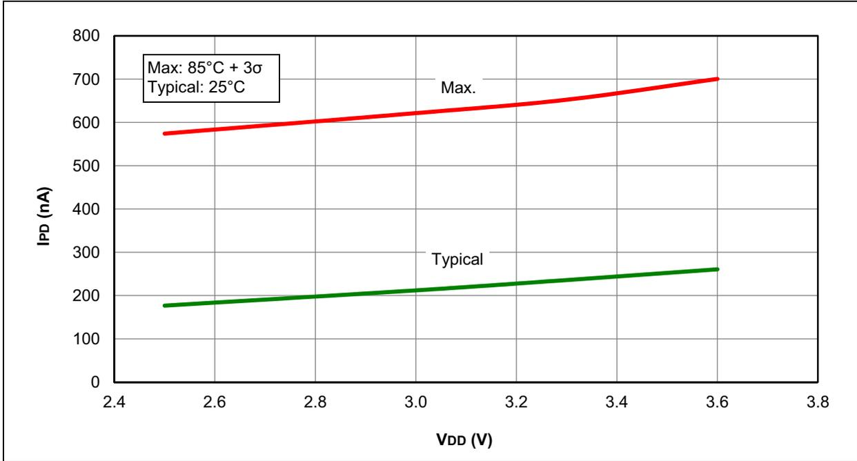
**FIGURE 31-8: I<sub>PD</sub>, LOW-POWER BROWN-OUT RESET (LPBOR), PIC16F1782/3 ONLY**
