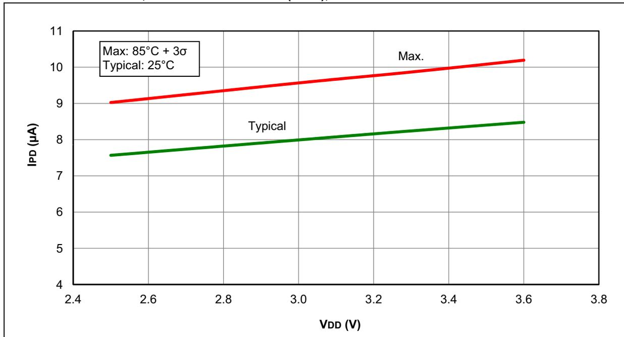
FIGURE 31-6: I<sub>PD</sub>, BROWN-OUT RESET (BOR), PIC16F1782/3 ONLY
