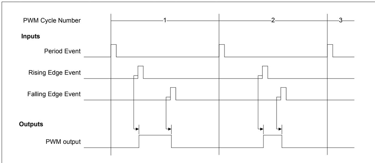
Each of the three types of events is triggered by a user selectable combination of synchronous timed and asynchronous external inputs.
