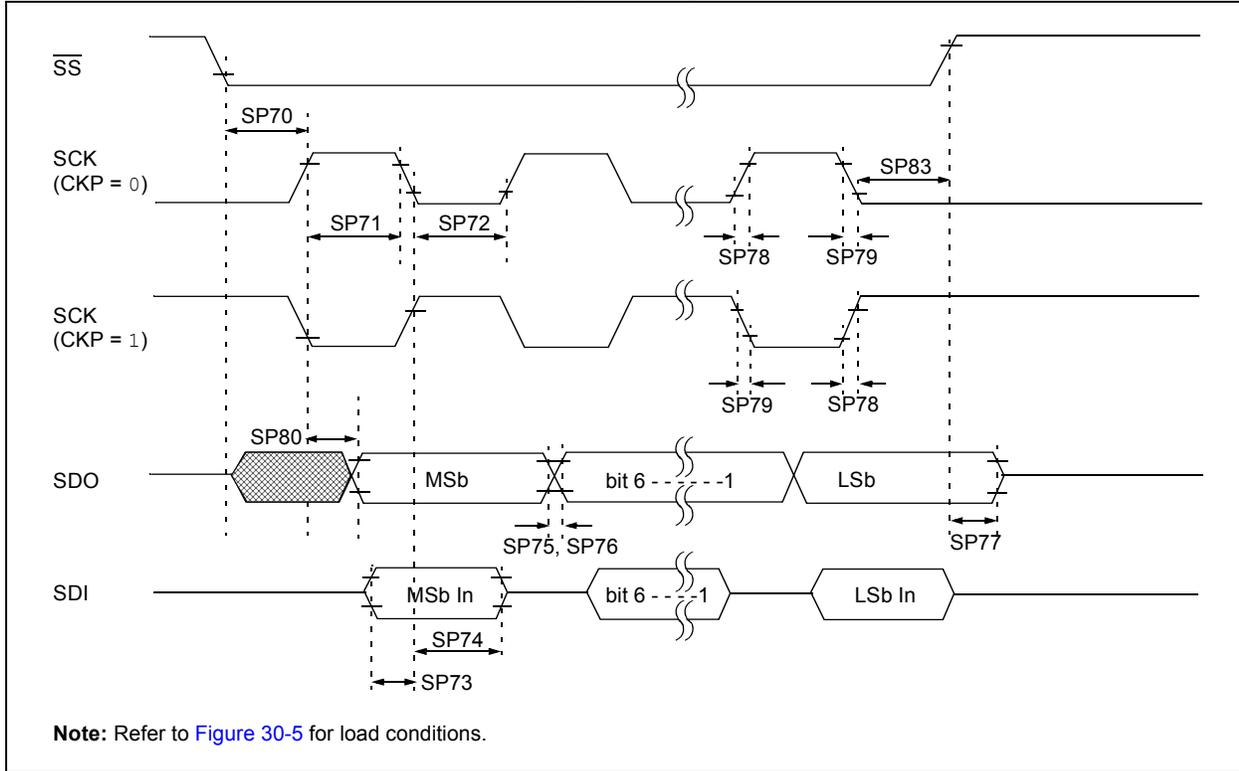
**FIGURE 30-19: SPI SLAVE MODE TIMING (CKE = 1)**
