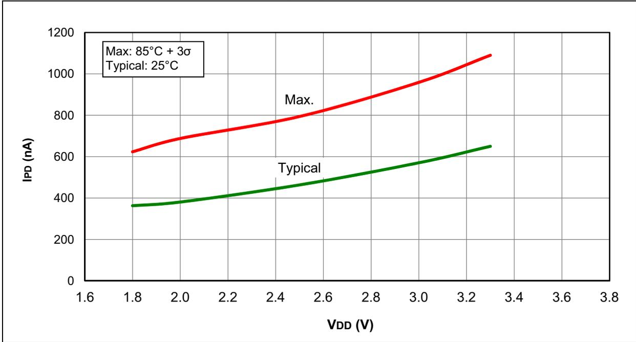
**FIGURE 31-4: I<sub>PD</sub>, WATCH DOG TIMER (WDT), PIC16F1782/3 ONLY**
