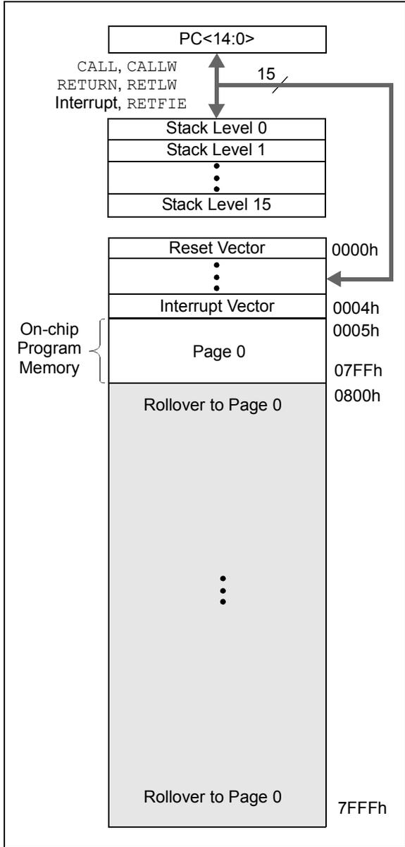
**FIGURE 3-2: PROGRAM MEMORY MAP AND STACK FOR PIC16F1783**
