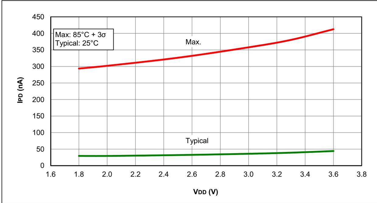
FIGURE 31-2: I<sub>PD</sub> BASE, LOW-POWER SLEEP MODE (VREGPM = 1), PIC16F1782/3 ONLY
