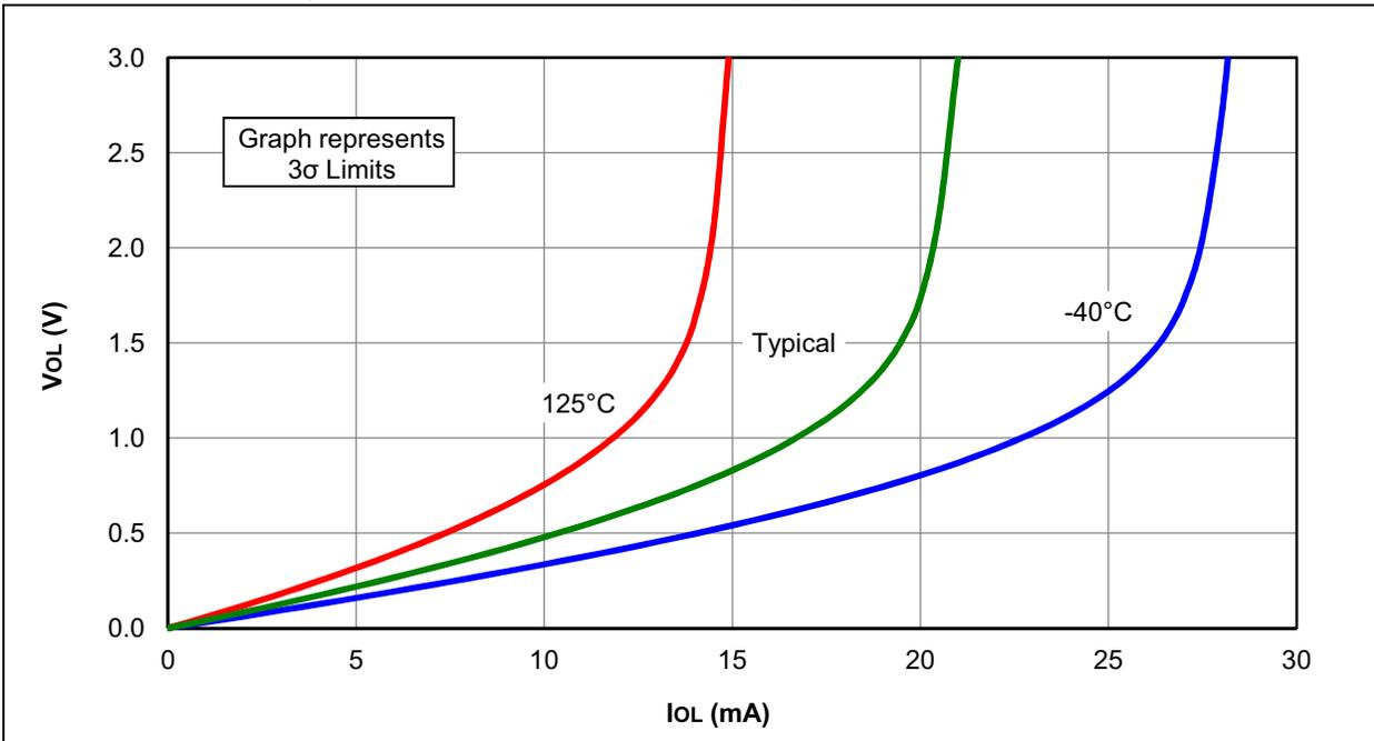
**FIGURE 31-15: I<sub>PD</sub>, V<sub>OL</sub> vs. I<sub>OL</sub> OVER TEMPERATURE, V<sub>DD</sub> = 1.8V, PIC16LF1782/3 ONLY**
