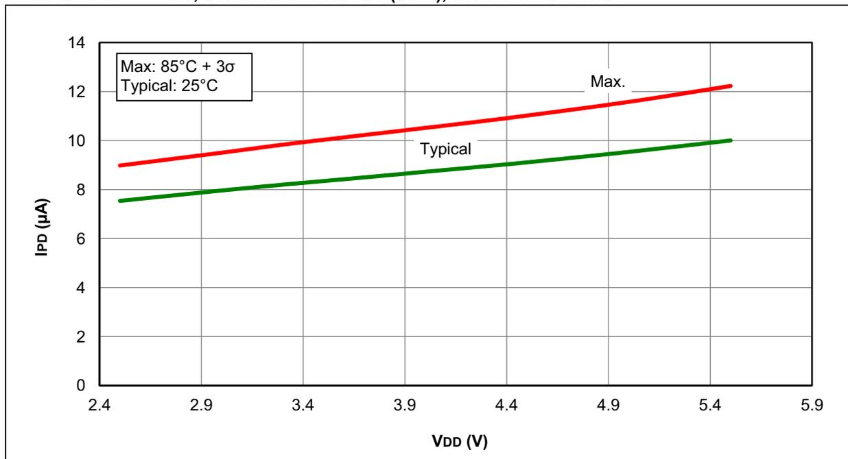
**FIGURE 31-7: I<sub>PD</sub>, LOW-POWER BROWN-OUT RESET (LPBOR), PIC16LF1782/3 ONLY**
