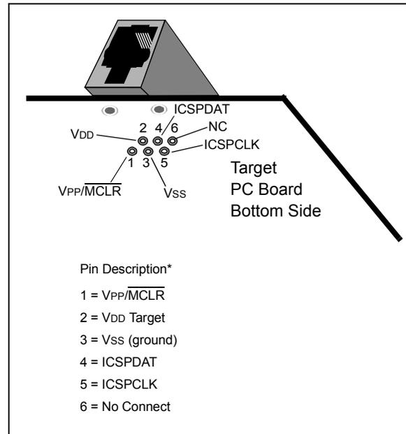
Another connector often found in use with the PICkit™ programmers is a standard 6-pin header with 0.1 inch spacing. Refer to Figure 28-2.
