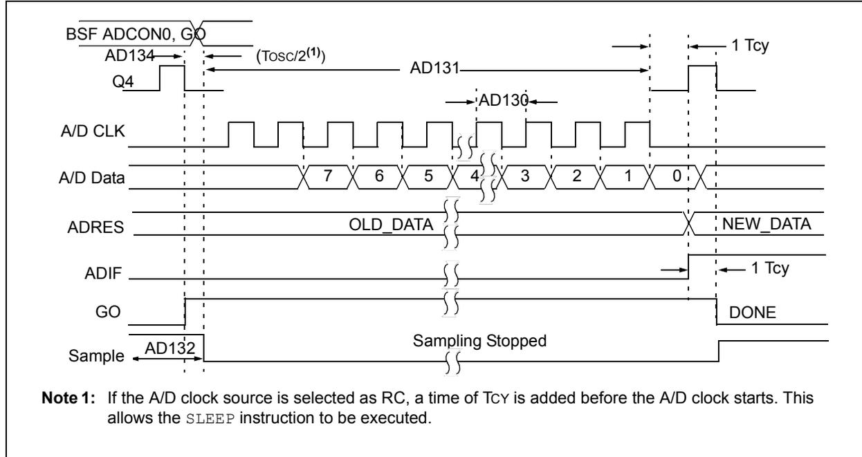
**FIGURE 30-13: PIC16(L)F1782/3 A/D CONVERSION TIMING (SLEEP MODE)**
