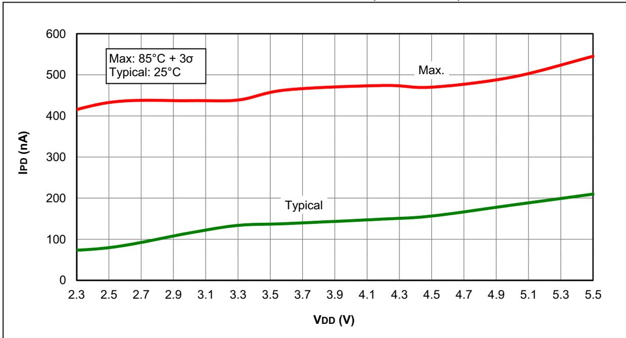
**FIGURE 31-3: I<sub>PD</sub>, WATCH DOG TIMER (WDT), PIC16LF1782/3 ONLY**
