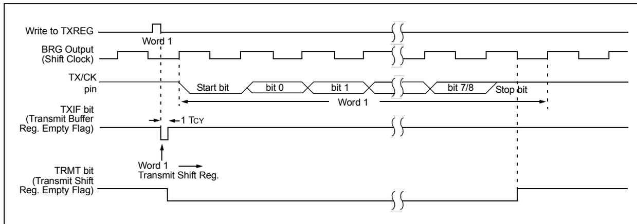
**FIGURE 27-4: ASYNCHRONOUS TRANSMISSION (BACK-TO-BACK)**
