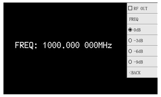
**[SIGNAL GENERATOR]** JNCRadio VNA 3G supports simple signal generator function, which can be set as a single-frequency continuous wave generator with a frequency range from 50kHz to 4400MHz. RF power is adjustable above 135MHz.
