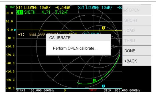
**NOTE**: usually we need to connect the DUT to VNA with cables, at this time, the cable becomes a part of the measurement system, and the end of the cable should be treated as the VNA port during calibration.
