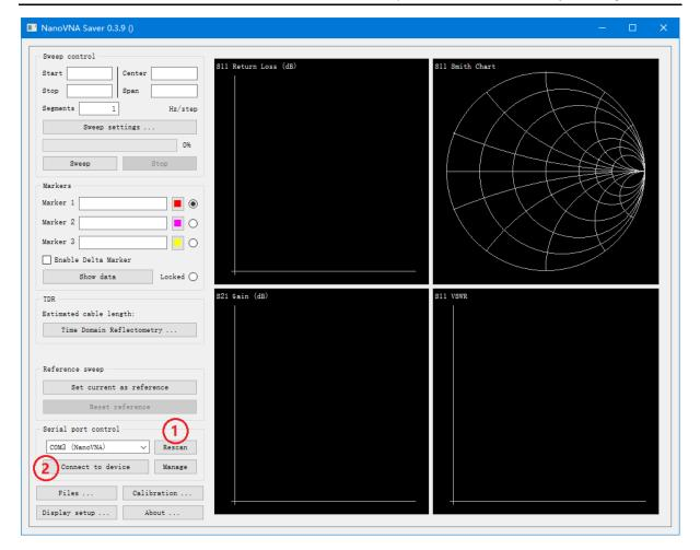
Through the PC software, you can set the start and stop frequency, get the measurement results, set the marker, take a screenshot, etc.
