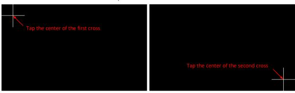
**Note:** After completing the calibration of the touch screen, you **MUST** execute saveconfig command to save the calibration data.
