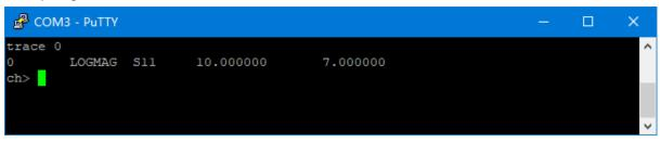
For the case of two parameters, the first parameter indicates to the trace number, the second parameter indicates to the trace format (logmag, phase, smith, linear, delay, swr).
