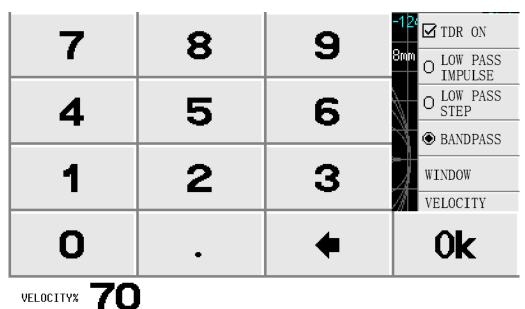
**NOTE**: Use a lower frequency to measure a longer length and a higher frequency to measure a shorter length and adjust accordingly for accurate results.
